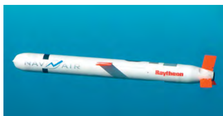
The Tomahawk cruise missile is being used to strike ISIS targets with remarkable accuracy using GPS (Global Positioning System) technology. On-board cameras allow the operator to determine its flight trajectory and its impact on the target
