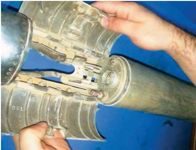
Russian Vypel NPO R-77 AAM and 'seeker head of the missile
