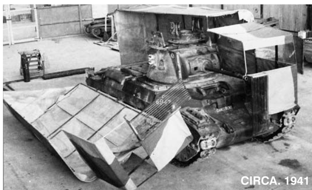
A tank disguised as a truck using a frame known as Sunshield. Middle East Command Camouflage Development and Training Centre, Helwan, Egypt
