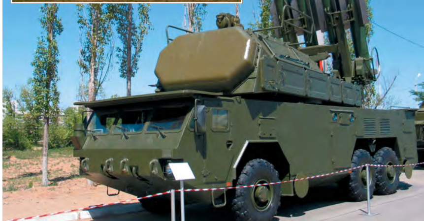
BUK-M (SA-11) mobile missile firing system
