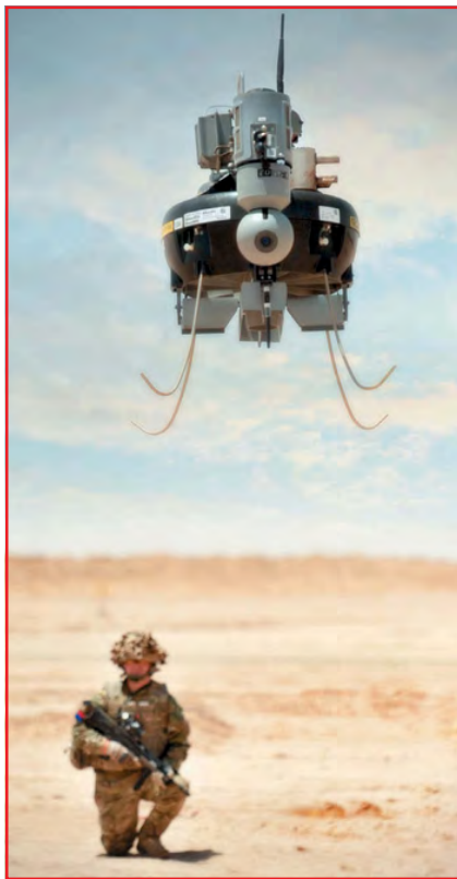
A British soldier watches a Tarantula Hawk (T-Hawk) Micro Remote Piloted Air System (RPAS) hover over the desert in Afghanistan. A special unit known as Talisman (counter-IED) uses the T-Hawk to check for roadside bombs and clear routes for large convoys
