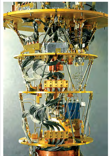
Support structure for installation of the D-Wave Vesuvius processor - NASA Quantum Artificial Intelligence Laboratory (QuaAIL)
