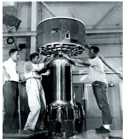
NASA's Tiros 1 weather satellite being shaken during a test to see if it will survive the violent ride into space in 1960
