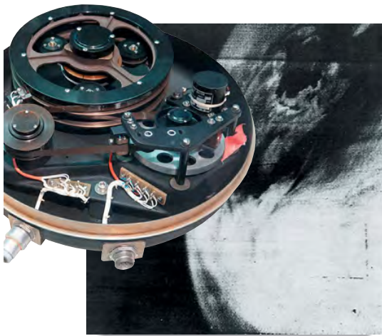
First television space image of Earth. Tiros-1 magnetic tape data recorder
