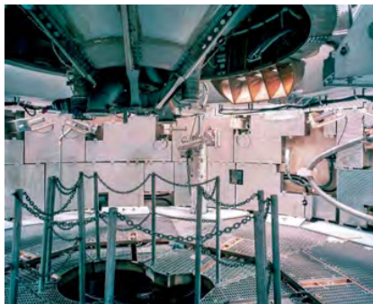
Titan II missile seven storeys below the surface. The two-stage booster can lift over two tons into low orbit and were also used for Gemini manned space missions
