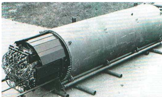
Cable tapping device built by AT&T Bell Laboratories
