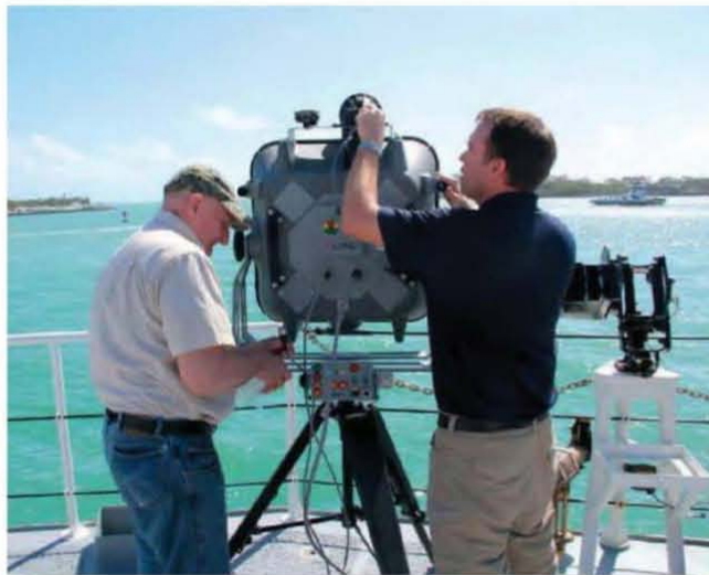
The DOD's JNLWD is developing a range of non-lethal weapons and acoustic devices. Above is the LRAD Hailing Acoustic Laser Light Tactical System appropriately called CG-HALLTS
