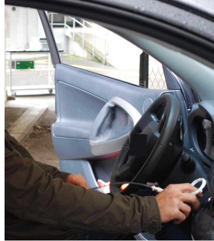
(b) Starting the engine using the relay.
