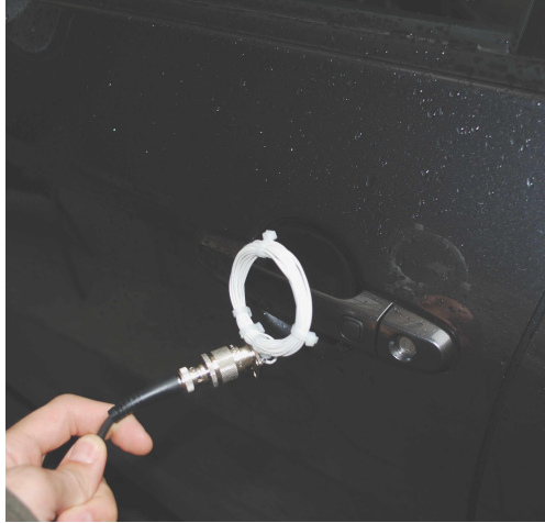
(a) Loop antenna placed next to the door handle.
