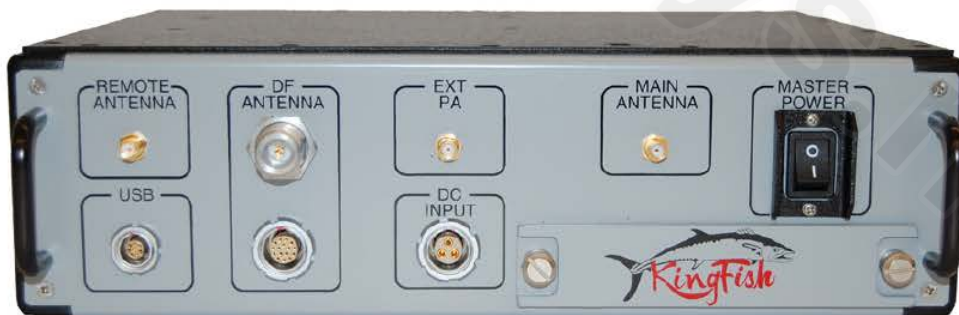
Figure 4-1. KingFish Front Panel
