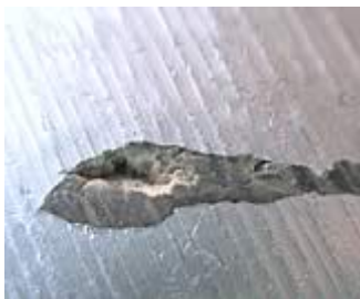
Wood: Melted into the center of an aluminum bar.
