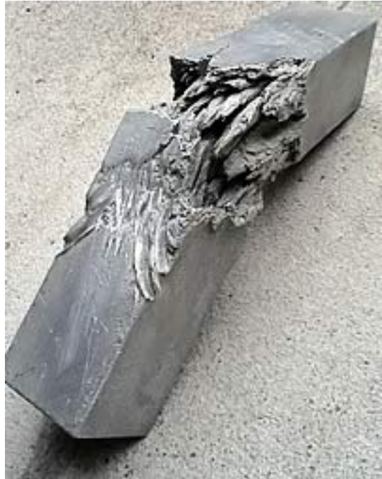
Aluminum Bar: The massive crack in the center is from a partial-jellification effect.
