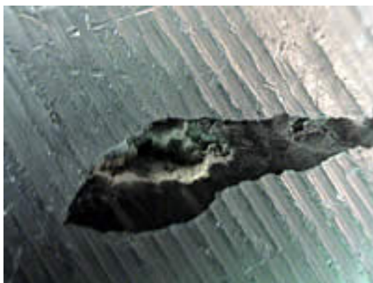
Wood: An extreme close-up shows that the wood has been 'welded' into the metal!
