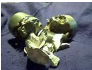
Rod: The center had been pulverized into a powder.
