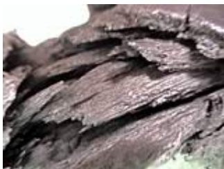
Extrusion: Close-up view of the deformed aluminum
