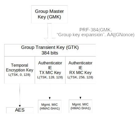
Figure 8—Complete WRAP Group Key Hierarchy for use with Authenticator IE
