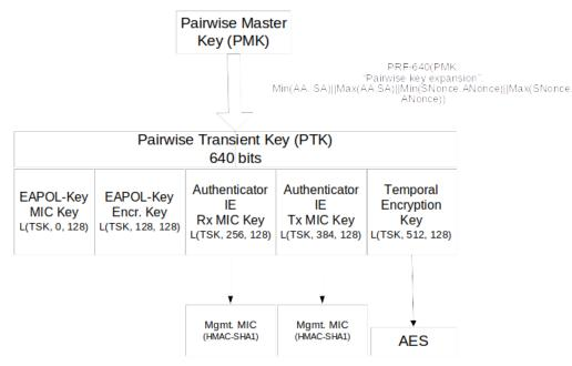
Figure 6—Complete WRAP Pairwise Key Hierarchy for use with Authenticator IE
