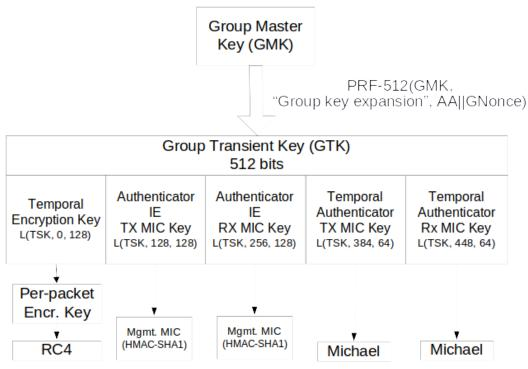
Figure 7—Complete TKIP Group Key Hierarchy for use with Authenticator IE
