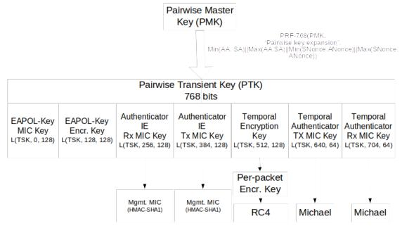
Figure 5—Complete TKIP Pairwise Key Hierarchy for use with Authenticator IE
