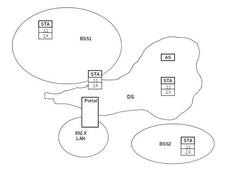
Figure 1: A robust security network (RSN)
