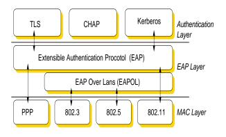
Figure 3: The EAP stack
