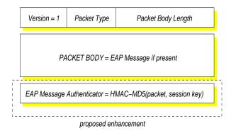
Figure 12: The changes to EAPOL: addition of an EAP authenticator attribute.
