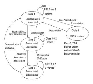
Figure 11: The 802.11i Robust Security Network state machine.
