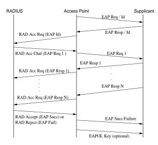
Figure 7: A complete 802.1X authentication session showing the EAP and RADIUS messages.
