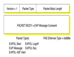
Figure 13: The EAPOL packet format.
