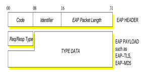
Figure 4: The EAP Packet.
