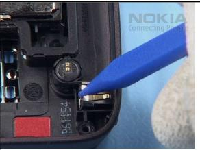
6. and push it carefully into place with the SS-93. Do not bend the spring contacts.
