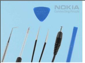
1. Needed tools: a Torx Plus size 6 screwdriver, metal tweezers, a DC plug, the SS-93 opening tool, a dental pick and the SRT-6.
