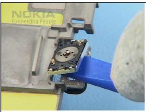
remove the EARPIECE ADHESIVE residues before assembling a new EARPIECE with a new EARPIECE ADHESIVE.
