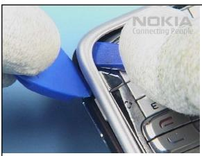
Hold the SS-93 in the shown position and unlock the side clip with SRT-6 by pressing it between the A-COVER and the B-COVER.
