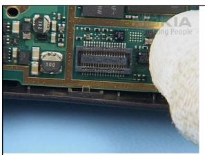
16. Secure the ENGINE MODULE.
