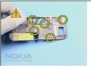
33. Gently, unlock the BASEBAND GASKET as shown and remove 34. Replace the EARPIECE when necessary. Keep in mind to it from the UI FRAME.
