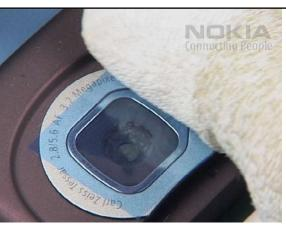
4. Cover the CAMERA WINDOW with a protective film.
