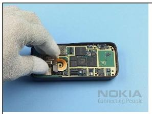
19. Insert the MAIN CAMERA into its housing...
