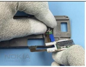
32. Move the UI MODULE to the primary position and then remove the UI MODULE by using the SS-93 as a support.
