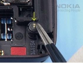
2. Insert the MICROPHONE exactly as shown, avoid bending the spring contacts.
