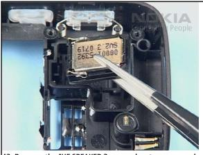
43. Remove the IHF SPEAKER 2 remember to remove whole IHF 44. Remove the MICROPHONE with the dental pick. GASKET 2 residues.
