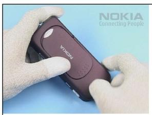
3. Unlock and open the SLIDE COVER ASSEMBLY.
