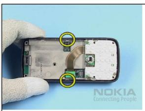
28. Put the UI FRAME into the B-COVER and press it into place.
