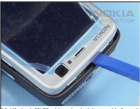
10. Lift the A-COVER a bit and unlock its top side from the B-COVER with the SS-93.
