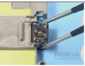
22. Place the EARPIECE with a new EARPIECE ADHESIVE into its frame, avoid bending the spring contacts.
