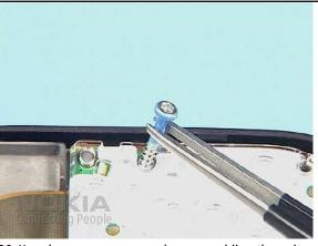
30. Use always new screws when assembling the unit.
