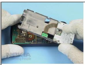
28. Remove the UI FRAME with the UI MODULE from the B-COVER.
