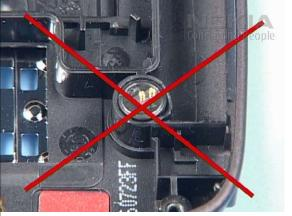
4. to avoid short-circuit or malfunction of the MICROPHONE..
