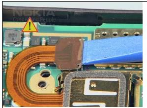
35. Disconnect the MAIN CAMERA from the ENGINE MODULE and 36. The ENGINE MODULE is snapped to the B-COVER with two remove it carefully from its housing.
