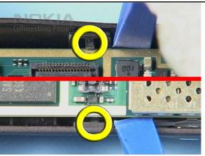
snaps. Unlock the ENGINE MODULE with the SS-93 ...
