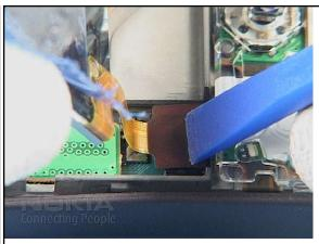
36. Connect the DISPLAY to the ENGINE MODULE...
