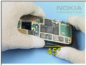
14. Insert the ENGINE MODULE under the shown angle.
