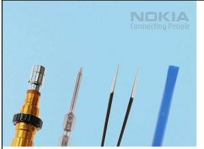
1. Needed tools: a Torque driver, a Torx size 6 plus bit, metal tweezers and the SS-93 opening tool.
