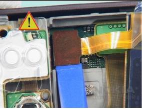
16. ...and disconnect it from the ENGINE MODULE.
