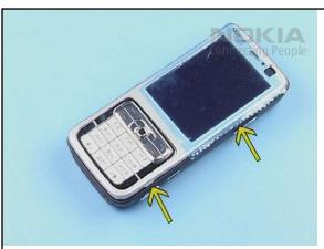
8. Slide the SRT-6 along the marked edges to unlock the snaps.
