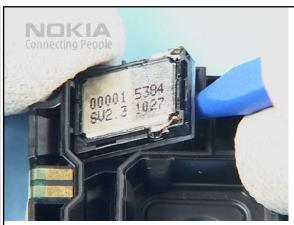
40. Lift the IHF SPEAKER from its housing and remove it easily.
