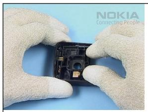
11. Insert the ANTENNA MOULDING in the B-COVER...
