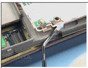
26. Lift the UI FRAME a bit and unsnap the LIGHT GUIDE.
