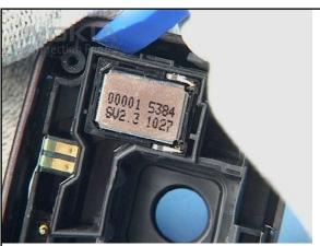
38. Unlock the ANTENNA MODULE ASSEMBLY with the SS-93 ...
