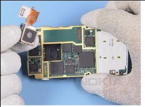
22. Check the camera and the window for cleanness before going on.
