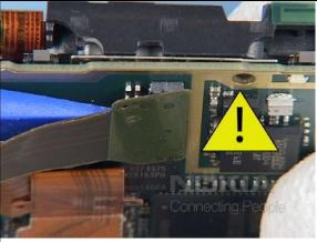
16. Be double careful while opening this connector. Do not destroy the hidden components underneath.
