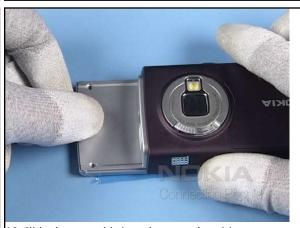
18. Slide the assembly into the second position to access the next treads.
