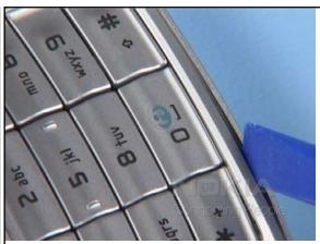
8. Gently pry open both plastic clips of the ITU KEYPAD.
