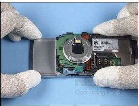
14. Shift out the assembly in order to gain the maximum flex foil length.
