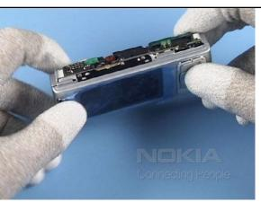
10. Shift the assembly together and turn it to access the screws.
