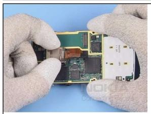
23. Position the MAIN CAMERA over its recess.
