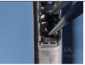
2. Fit a new gasket and place the EARPIECE into the FRONT COVER.
