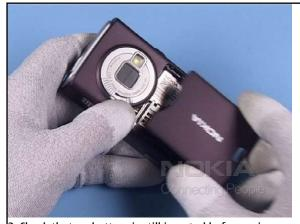
3. Check that no battery is still inserted before going on.
