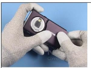
3. Unlock and remove the BATTERY COVER.
