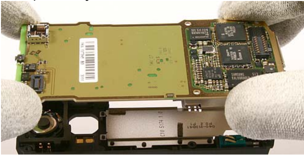
25.) Remove the Engine Module . Place it into the RJ-94 jig immediately.
