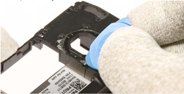
33.) Remove the residues of the Camera Rear Bezel Assy Adhesive completely with the SRT-6. For assembly always use a new adhesive.
