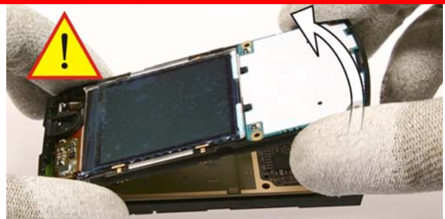
16.) Lift the UI-frame Assy from Chassis Assy . Mind the still connected flex foil of the LCD.
