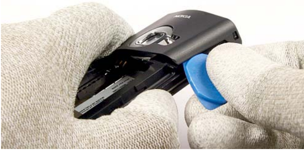
9.) Insert the SRT-6 between the Antenna Cover and Chassis Assy . Additional force may be required while opening the Antenna Cover clips.
