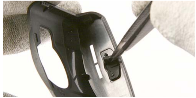
10.) Remove the Power Button with tweezers.
