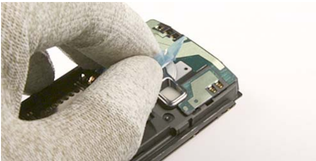
11.) Protect the Camera Rear Bezel Assy with a plastic film before turning the unit.
