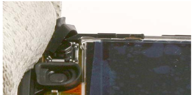
12.) Remove the Camera gasket .
