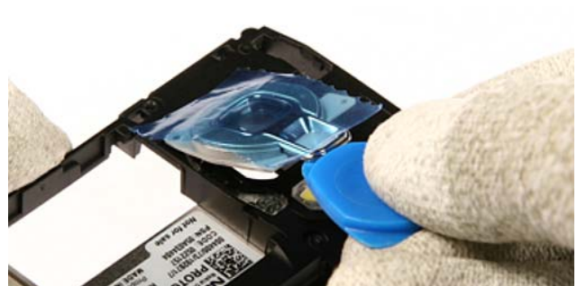
32.) Lever out the Camera Rear Bezel Assy .
