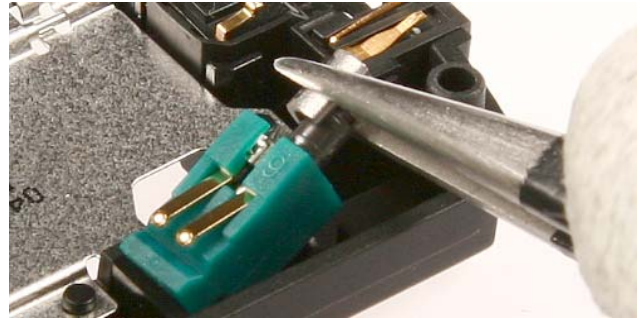
26.) Remove the Vibra Motor with tweezers.
