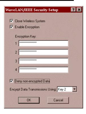
This figure shows how the read-back screen would appear when four keys were entered and Key2 selected as transmit key.
