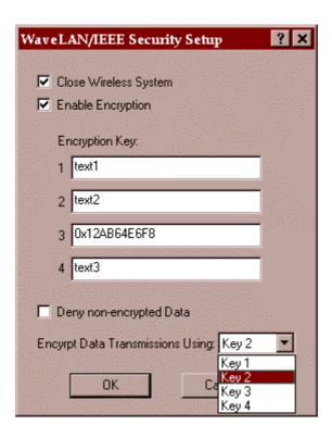
One to four encryption keys must be entered when the Enable Encryption selection is done. These keys will be used to encrypt or decrypt data transmissions. The format of entering the key values is either in textual format or in hexadecimal format (an entry starting with "0x" will be interpreted as hexadecimal). A text string is translated in the ASCII values associated with each character.
