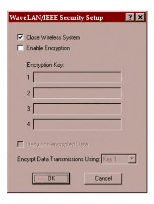
The tick-box "Close Wireless System" is not related to WEP encryption and is not further covered.
