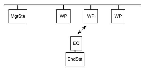
As long as the network is WEP protected, the reconfiguration information (including new keys) can be transmitted over the ethernet and the wireless path via the WP units that connect the EC units. This way, the EC units can be reconfigured from a central location.
