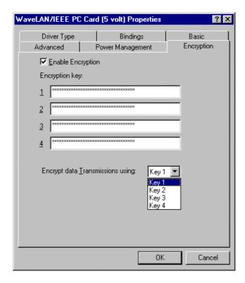
The configuration at the station side has similar parameters as for the WavePOINT, with the exception of the "Deny Non-encrypted Data" tick-box. In a station it will always be possible to receive non-encrypted data. The primary example where this is useful is for the reception of non-encrypted multicast messages as will be required in a mixed system.
