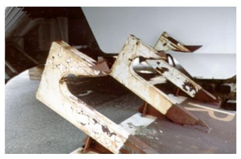
Picture 16. The two middle hooks seen here have been severe damaged.
