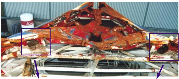
Picture 20. Overview of the bottom plate damage and details below.
