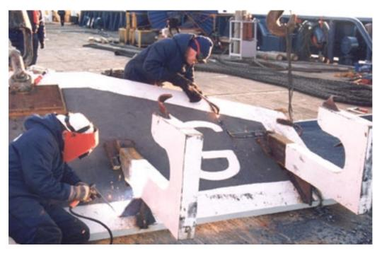
Picture 9. The picture shows the fourth redesign. It involved removing major parts of the upper corners of the yoke by means of cutting, and also cutting away material on each side of the yoke to make it narrower.
