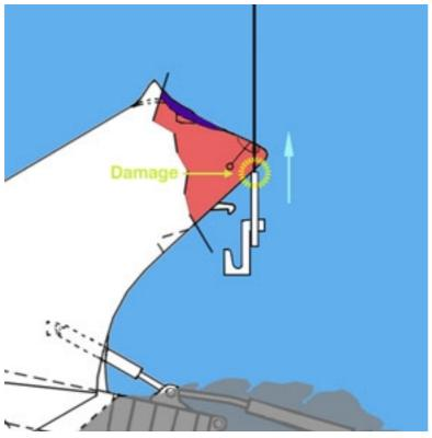
Damage type one. Damage from the yoke due to failure to attach it to the visor (dimensioning problems). The yoke may have hit the visor in several places.
