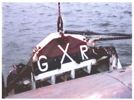
Picture 11. The visor emerging from the water.
