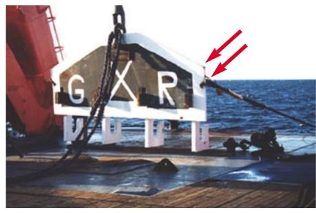
The fastening points have been cut off moved down and slightly. The second design are shown here in picture 7.
