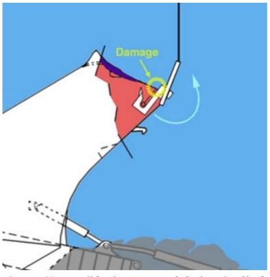
Damage type four. Damage from the yoke after it was forced to attach to the visor. When the visor was lifted it was damaged due to bending force. This caused further separation between the transverse beams and the plating and may also have damaged the visor bottom plating further.
