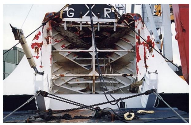
Picture 6. The yoke (marked G X R) hooked into the visor after recovery.
