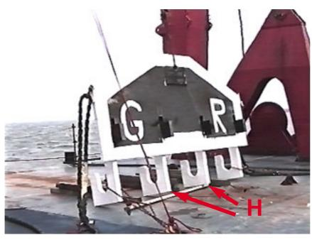
The recovery plan was to lower the yoke in the sea down to the visor and then "catch" the visor with the hooks. The operation was to be monitored by a (Sjöugglan) and control of the ROV was manned on the Furusund. The theory of the "catch" is described in picture 5 on the next page. It can also be compared with picture 6 which shows the yoke hooked to the visor after the visor was recovered to the surface.
