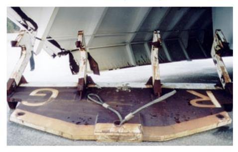
Picture 15. Three hooks are damaged. The outer port side hook, to the right of the picture, was not damaged.
