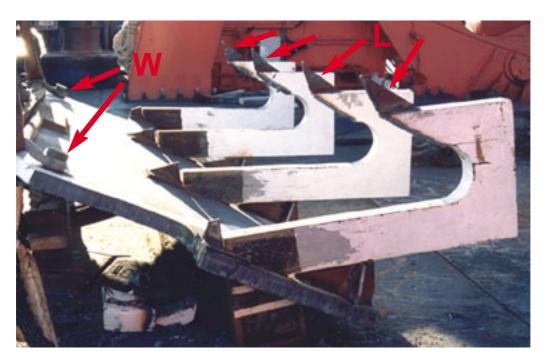
Picture 10. The picture shows the result of the fourth redesign. Material from the hooks was also cut away, and the relative angle between the yoke and the hooks was changed. New holes were cut for the two wires or thick ropes (W) that were attached on each side of the yoke. The triangular lugs on the hooks have been repaired (L).
