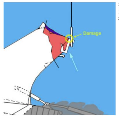
Damage type three. Damage from the yoke as it was forced to attach to the visor beam.
