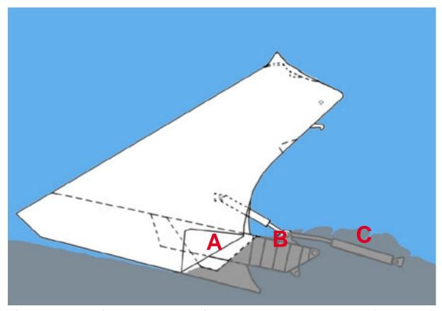
Picture 1. The picture shows the visor seen from the starboard side, standing upside down resting on the visor housing (A) with the visor arms (B) and the starboard hydraulic actuator (C) covered with mud. On the video (visiri) it can be seen that the rest of the visor was standing free from the bottom and that there were no contact marks on the bottom around the front of the visor.
