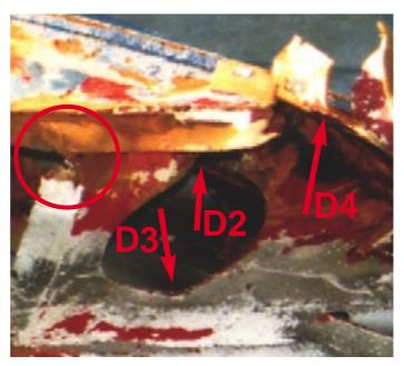
Picture 22. The round hole is damaged (D2) in an forward direction. The outer port hook on the yoke has broken the plate with the hole when twisting around the transverse tube beam. It has also created buckling (D3). The yoke also broke the beam (D4) as can also be seen in picture 23.
