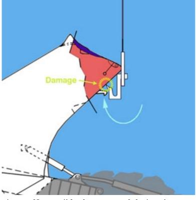
Damage type two. Damage from the yoke as the modified hooks with sharp lugs hit the visor. The lugs were bent as a result of hitting the visor. Score marks must have been caused. The hooks may also have ripped and damaged other parts of the visor.
