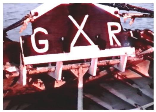
Picture 12. The hooks on the redesigned yoke attached to the transverse visor beam slid slightly towards the starboard side of the visor.
