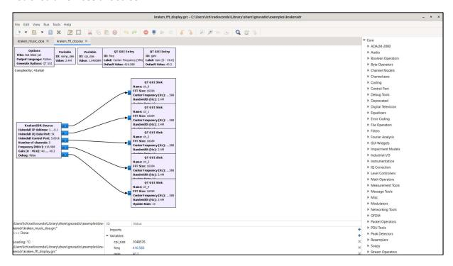
Double-click on the KrakenSDR Source block to the left and replace the default Heimdall IP address 127.0.0.1 with the Pi's Ethernet IPV4 address 169.254.24.100.
