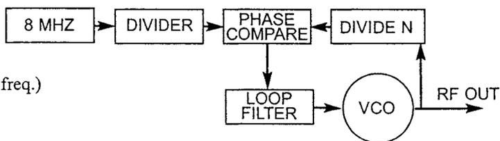
In the example below we will use a 8 mhz crystal, a reference of 100 khz and the RF frequency we will lock to is 99.9 mhz. The reference divider is 80 and the RF divider is 999.
