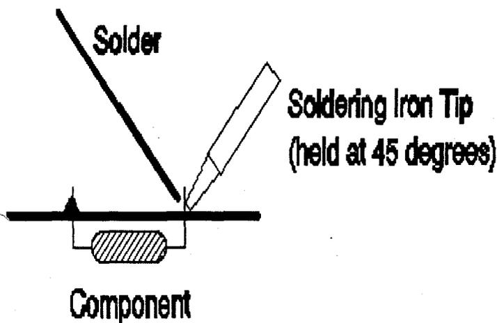
to the tip of the cone as possible. **Important.** In R.F. construction, solder components as close to the board as possible, unless otherwise instructed, or the circuit will be prone to instability due to extra lead length adding spurious inductance and capacitance.
