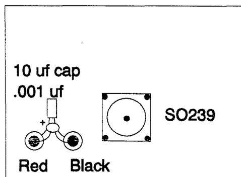
Follow the wiring diagram for the audio input. Two leads will go to the PLL board, audio in and ground. These can be either twisted pair or shielded 2 conductor cable.
