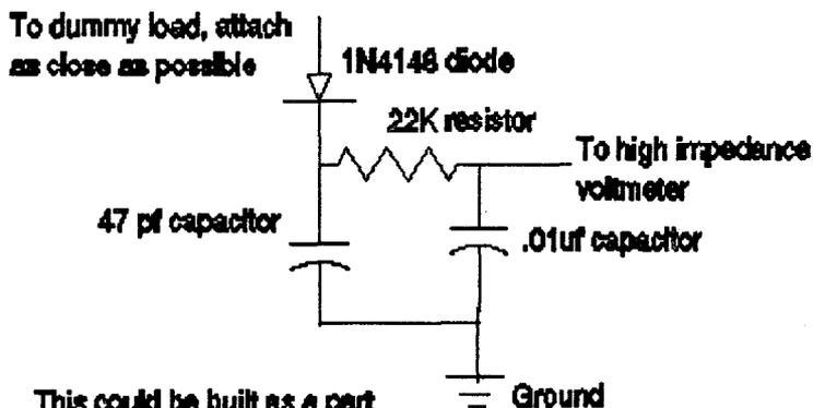
This could be built as a part of the dummy load shown in a previous diagram, keep lead lengths as short as possible
