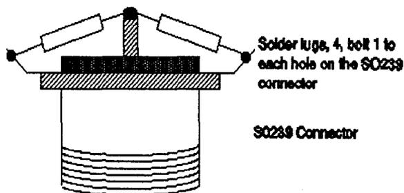
Solder lugs, 4, bolt 1 to each hole on the SO239 connector
