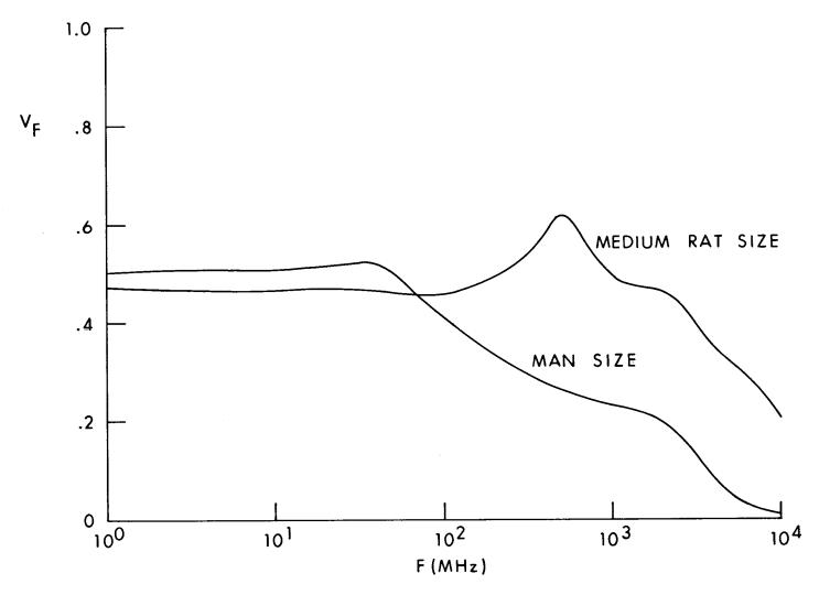
Figure 5.6. The volume fraction,  $V_{\rm F}$ , as a function of frequency for two spheres of muscle material.  $V_{\rm F}$  is the fraction of the volume in which 90% of the power is absorbed (see p. 5.15).
