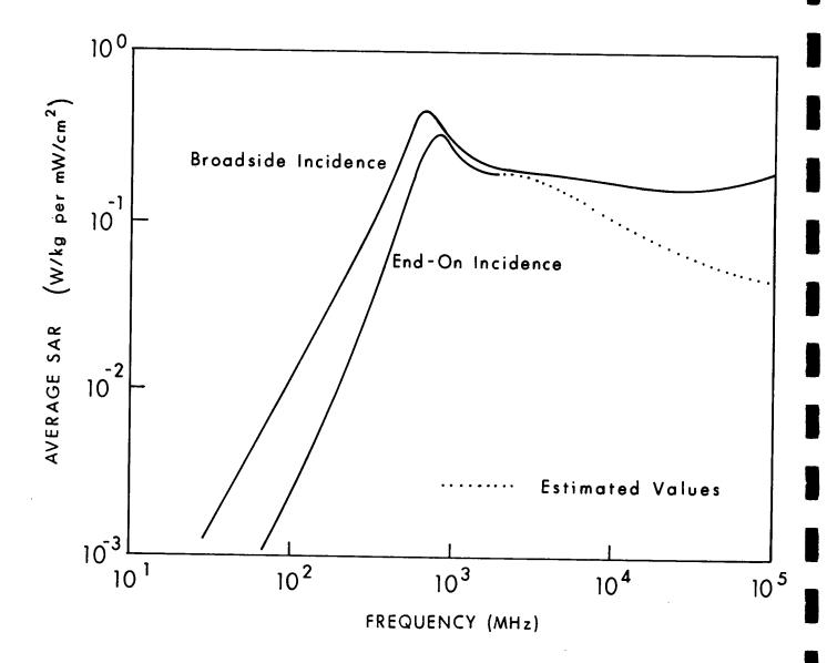
Figure 6.27. Calculated planewave average SAR in a prolate spheroidal model of a medium rat irradiated by a circularly polarized wave, for two orientations; a = 0.1 m, b = 0.0276 m,  $V = 3.2 \times 10^{-4} \text{ m}^3$ .
