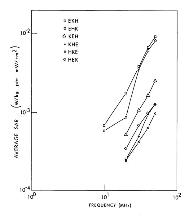
Figure 8.7. Measured values of the average SAR for saline-filled ellipsoidal phantoms, for six standard polarizations; a=20 cm, b=7.92 cm, c=5.28 cm,  $\sigma=0.36$  S/m (Allen et al., 1976).
