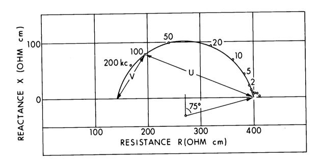
Figure 4.2. Dielectric properties of muscle in the impedance plane, with reactance X plotted against resistance R and the impedance Z = R + jX (Schwan, 1957). The large circle results from the  $\beta$ -dispersion and the small one from the  $\alpha$ -dispersion. The plot does not include the  $\gamma$ -dispersion.
