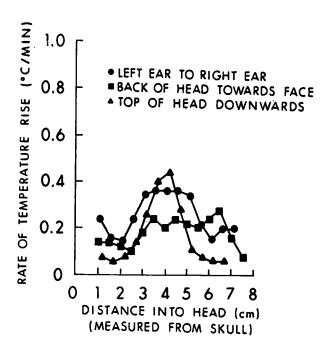
Figure 8.25. Rate of temperature rise from RFR exposure in the face of a detached M. mulatta head; 1.2 GHz, CW, 70 mW/cm<sup>2</sup>, far field (Burr and Krupp, 1980).
