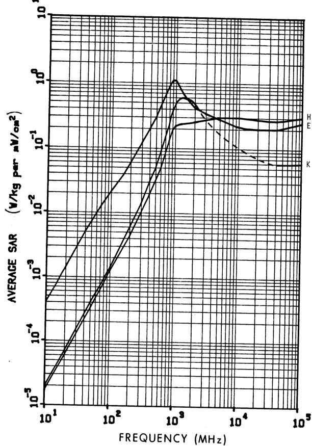
Figure 6.15. Calculated planewave average SAR in a prolate spheroidal model of a small rat for three polarizations; a=0.07 m, b=0.194 m,  $V=1.1\times10^{-4}$  m<sup>3</sup>. The dashed line is estimated values.
