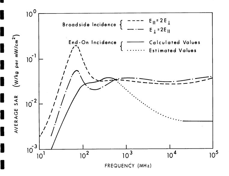
Figure 6.28. Calculated planewave average SAR in a prolate spheroidal model of an average man irradiated by an elliptically polarized wave, for two orientations; a=0.875 m, b=0.138 m,  $V=0.07 \text{ m}^3$ .
