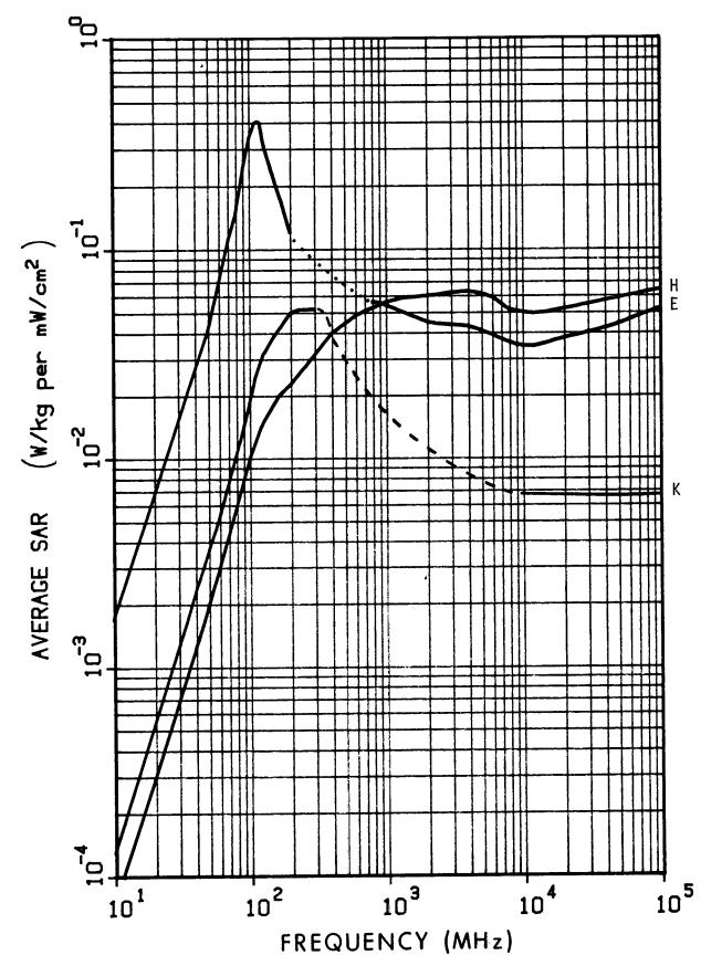
Figure 6.8. Calculated planewave average SAR in a prolate spheroidal model of a 5-year-old child for three polarizations; a=0.56 m, b=0.091 m, V=0.0195 m<sup>3</sup>. The dotted line is calculated from Equation 5.1; the dashed line is estimated values.
