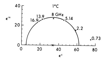
Figure 4.3. Dielectric properties of barnacle muscle in the microwave frequency range are presented in the complex dielectric constant plane (Foster et al., 1980).
