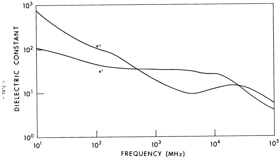
Figure 3.35. Average permittivity of the human body (equivalent to two-thirds that of muscle tissue) as a function of frequency.
