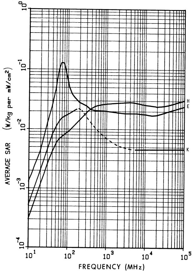
Figure 6.5. Calculated planewave average SAR in a prolate spheroidal model of an average endomorphic (fat) man for three polarizations; a = 0.88 m, b = 0.195 m, V = 0.141 m $^3$ . The dashed line is estimated values.
