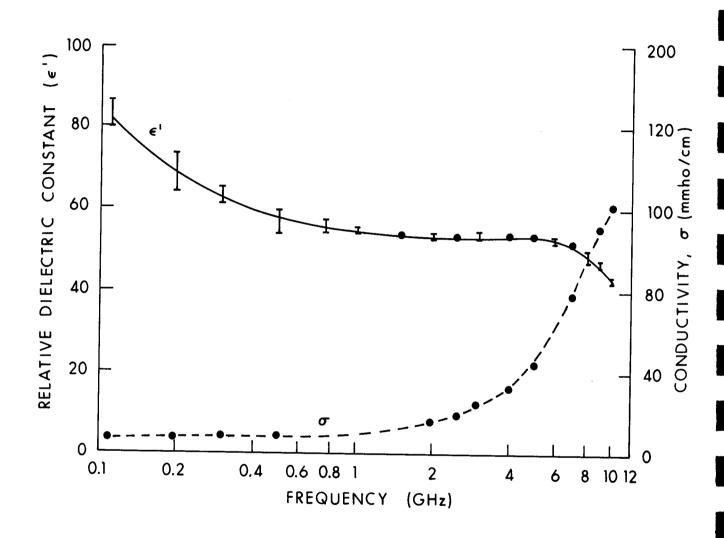
Figure 4.18. Measured values of relative dielectric constant and conductivity of in vivo rat brain at 32°C. Maximum SEM for  $\epsilon'$  is indicated by error bars and SEM for  $\epsilon''$  =  $\pm$  0.9 (Burdette et al., 1980).
