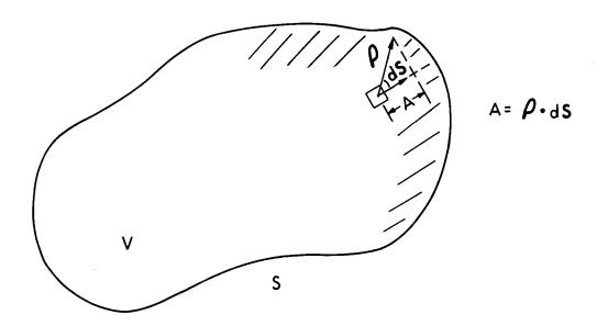
Figure 3.27. A volume (V) bounded by a closed surface (S). dS is the differential surface vector.  $\boldsymbol{\rho} \cdot d\mathbf{S}$  is the projection of  $\boldsymbol{\rho}$  on dS, which corresponds to power passing out through dS.
