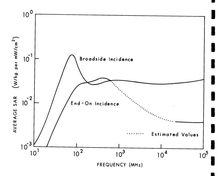
Figure 6.25. Calculated planewave average SAR in a prolate spheroidal model of an average man irradiated by a circularly polarized wave, for two orientations; a = 0.875 m, b = 0.138 m,  $V = 0.07 \text{ m}^3$ .
