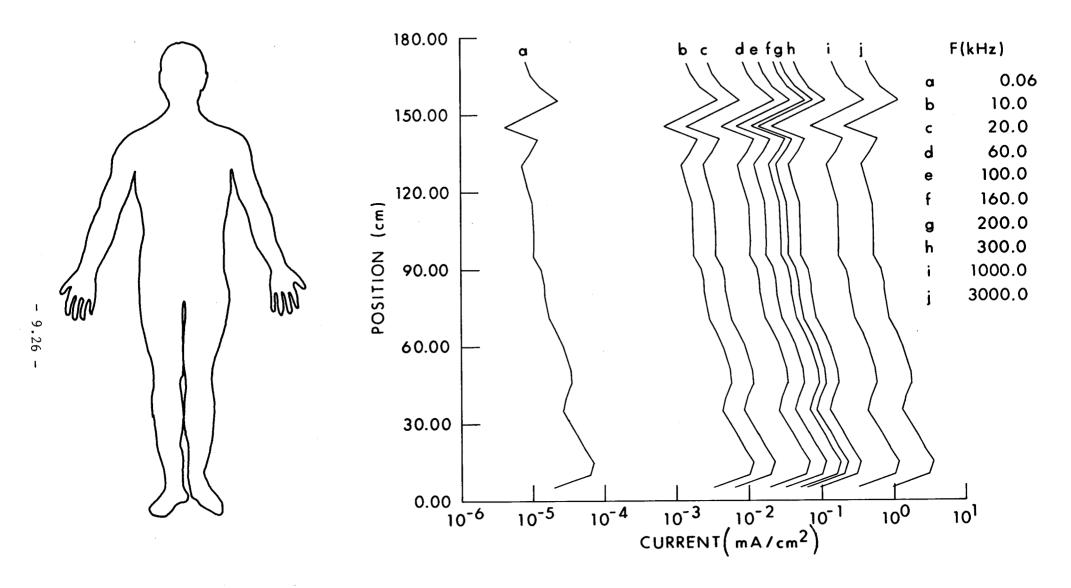
Figure 9.12. Calculated current distribution as a function of position in man exposed to 1-kV/m VLF-MF fields in free space (Guy and Chou, 1982).
