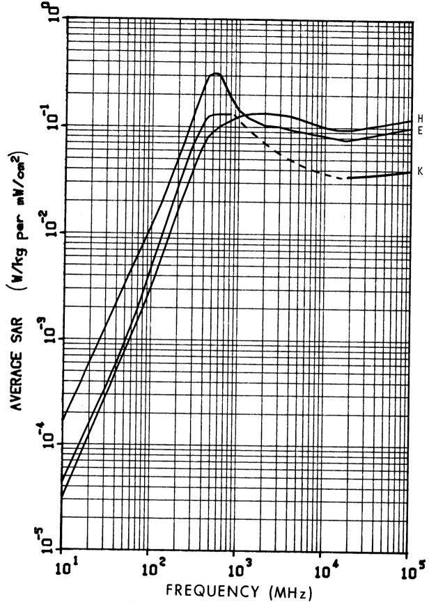
Figure 6.11. Calculated planewave average SAR in a prolate spheroidal model of a squirrel monkey for three polarizations; a = 0.115 m, b = 0.0478 m,  $V = 1.1 \times 10^{-3} \text{ m}^3$ . The dashed line is estimated values.
