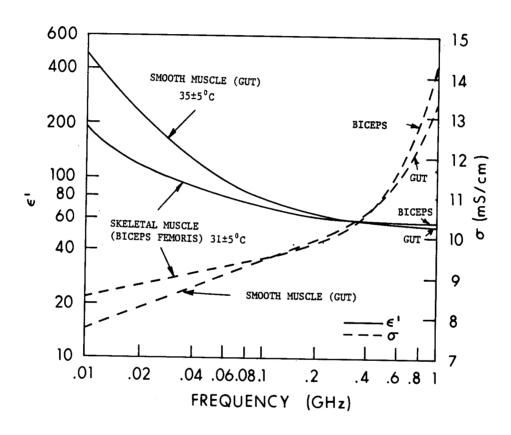
Figure 4.22. Average relative permittivity of two types of cat muscle in vivo (five samples for each point) (Stuchly et al., 1981).
