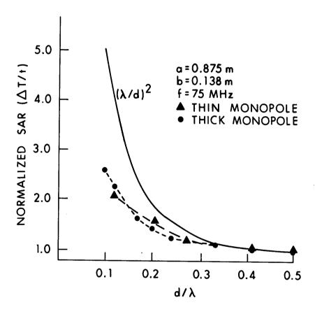
Figure 8.19. Measured relative SARs in scaled saline spheroidal models of man. To emphasize the differences in the absorption characteristics, the values are normalized with respect to their far-field value at  $d/\lambda = 0.5$ .  $\Delta T$  is the temperature rise in the saline solution after exposure for time t (Iskander et al., 1981).
