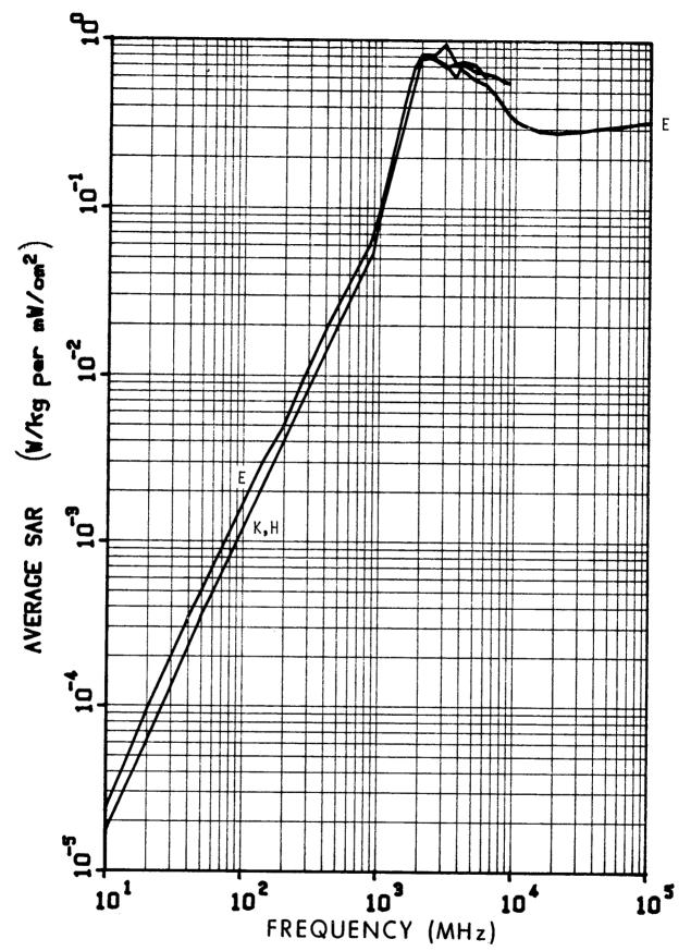
Figure 6.19. Calculated planewave average SAR in a prolate spheroidal model of a quail egg for three polarizations; a = 1.5 cm, b = 1.26 cm, and V = 10 cm<sup>3</sup>.
