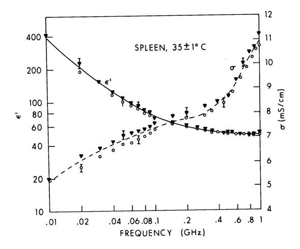
Figure 4.21. Relative permittivity of cat spleen in vivo: ▼ and ○ show results obtained for two locations; the vertical bars show the uncertainty due to estimated measurement errors (SD) (Stuchly et al., 1981).
