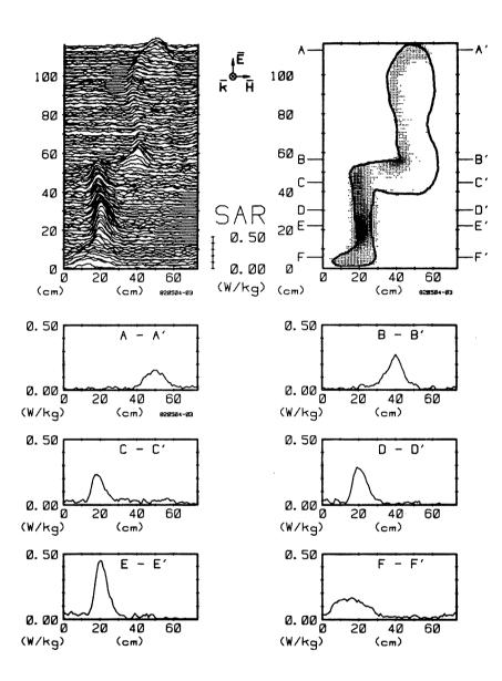
Figure 8.46. Computer-processed whole-body thermograms expressing SAR patterns for man sitting (sagittal plane through leg), exposed to 1-mW/cm<sup>2</sup> 450-MHz radiation with EHK polarization (Guy et al., 1984) (© 1984 IEEE).
