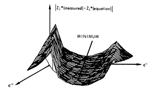
Figure 4.11. Graphical illustration of the iterative procedure for calculating complex permittivity parameters by minimizing the difference between measured and calculated values of the input impedance of the in vivo dielectric probe. The minimum on the error surface | Z measured - Z calculated indicates the most appropriate values of  $\epsilon$ ' and  $\epsilon$ " that satisfy the measured value of the input impedance.
