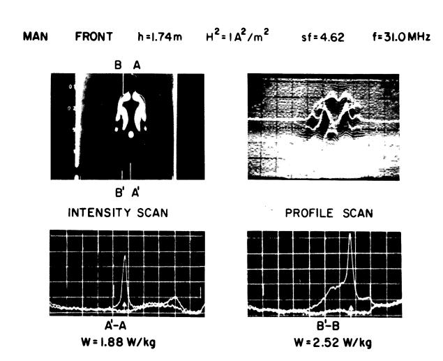
Figure 8.37. Scale-model thermograms and measured peak SAR for 70-kg, 1.74-m-height frontal-plane man model exposed to 31.0-MHz magnetic field perpendicular to the major axis: vertical divergence = 2°C, horizontal divergence = 4 cm (Guy et al., 1976b) (© 1976 IEEE).
