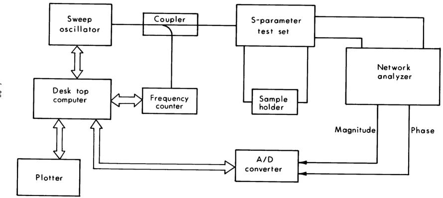
Figure 4.7. Experimental setup for measuring S-parameters, using an automatic network analyzer.
