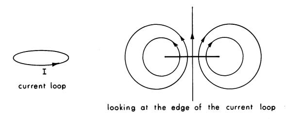
Figure 3.12. B-field produced by a circular current loop.
