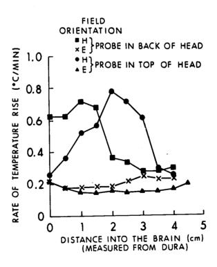
Figure 8.28. Rate of temperature rise from RFR exposure to the back of an M. mulatta cadaver head (with body attached); 1.2 GHz, CW, 70 mW/cm<sup>2</sup>, far field.
