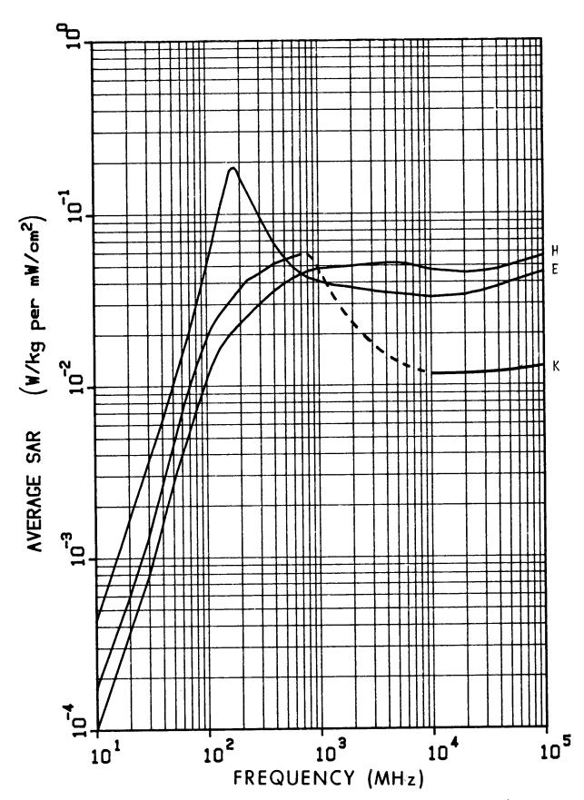
Figure 6.12. Calculated planewave average SAR in a prolate spheroidal model of a Brittany spaniel for three polarizations; a = 0.344 m, b = 0.105 m, V = 0.0159 m<sup>3</sup>. The dashed line is estimated values.
