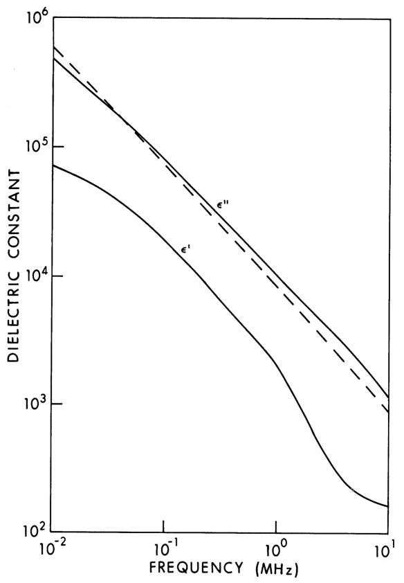
Figure 9.18. Real part,  $\epsilon'$ , and imaginary part,  $\epsilon''$ , of the dielectric constant for high-water-content tissue. The dashed line is measured values (Guy and Chou, 1982). The other lines are values given in the first edition of this handbook.
