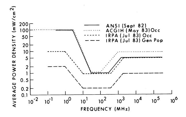
Figure 11.3. Comparison of RFR safety guidelines based on a threshold of 4 W/kg for adverse effects.
