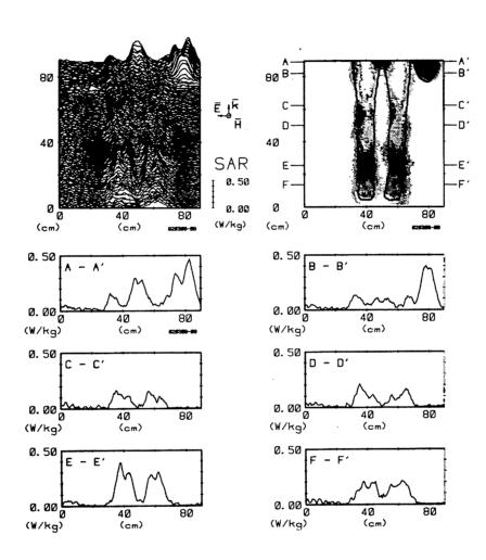
Figure 8.44. Computer-processed lower-body thermograms expressing SAR patterns for man with one arm extended, exposed to 1-mW/cm<sup>2</sup> 450-MHz radiation with KEH polarization (Guy et al., 1984) (© 1984 IEEE).
