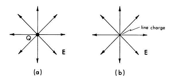
Figure 3.8. (a) E-field produced by one point charge, Q, in space.
