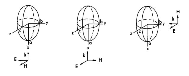
Figure 3.38. Polarization for objects that do not have circular symmetry about the long axis.
