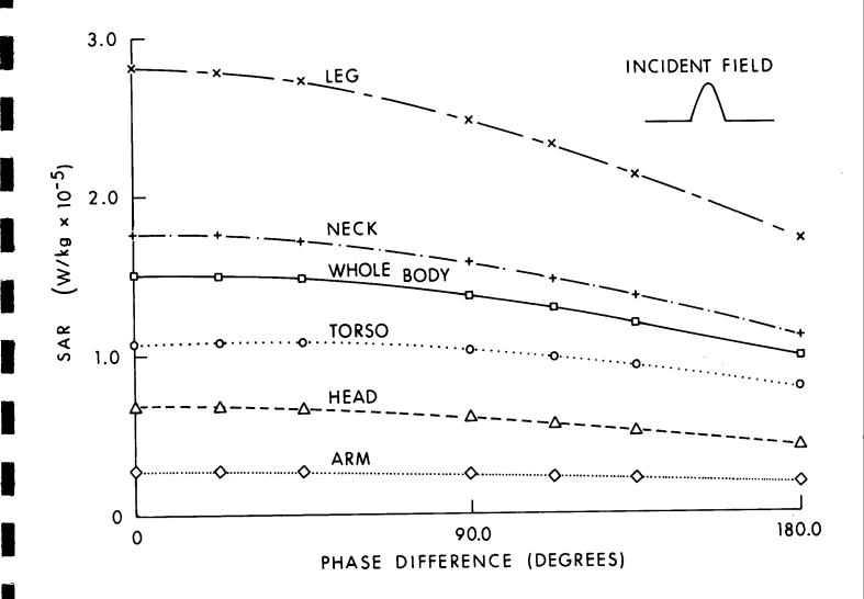
Figure 6.48. Whole- and part-body SAR at 77 MHz in the block model of man as a function of an assumed linear symmetric phase variation in the incident  $E_z$ ;  $E_z$  = 1 V/m. Calculated by Chatterjee et al. (1980a, 1980b, 1980c).
