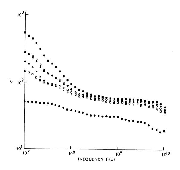
Figure 4.26. The real part of the dielectric constant, ε', of ocular tissues at 37°C (Gabriel et al., 1983).
