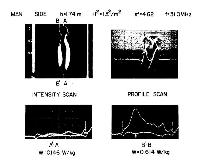
Figure 8.38. Scale-model thermograms and measured peak SAR for 70-kg, 1.74-m-height medial-plane man model exposed to 31.0-MHz magnetic field perpendicular to the median plane: vertical divergence = 2°C, horizontal divergence = 2.65 cm (Guy et al., 1976b) (© 1976 IEEE).
