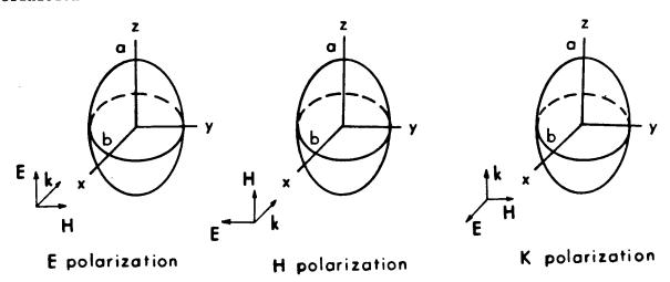
Figure 3.37. Polarization of the incident field with respect to an irradiated object.
