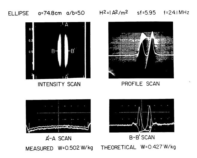
Figure 8.35. Scale-model thermograms and calculated peak SAR for 70-kg, 5/1 prolate spheroid (a = 74.8 cm) exposed to 24.1-MHz magnetic field perpendicular to the major axis: vertical divergence = 2°C, horizontal divergence = 2.65 cm (Guy et al., 1976b) (© 1976 IEEE).
