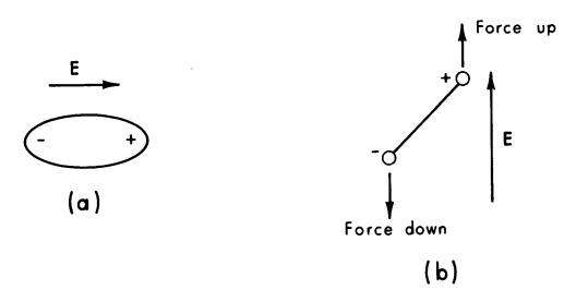
Figure 3.14. (a) Polarization of bound charges.
