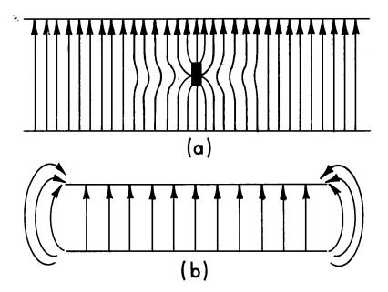
Figure 3.10. (a) E-field lines when a small metallic object is placed between the plates.
