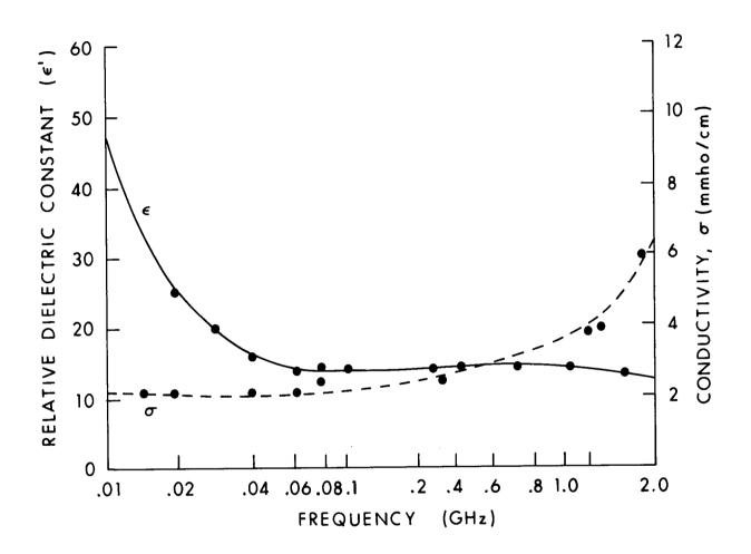
Figure 4.17. Measured values of relative dielectric constant and conductivity of in vivo canine fat tissue at 37°C (Burdette et al., 1980).
