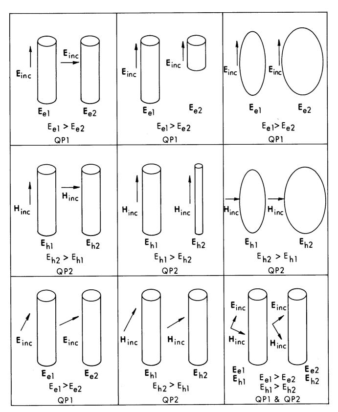
Figure 5.12. Qualitative evaluation of the internal fields based on qualitative principles QPl and QP2. E is the internal E-field generated by E, the incident E-field, and E is the internal E-field generated by H, the incident H-field.
