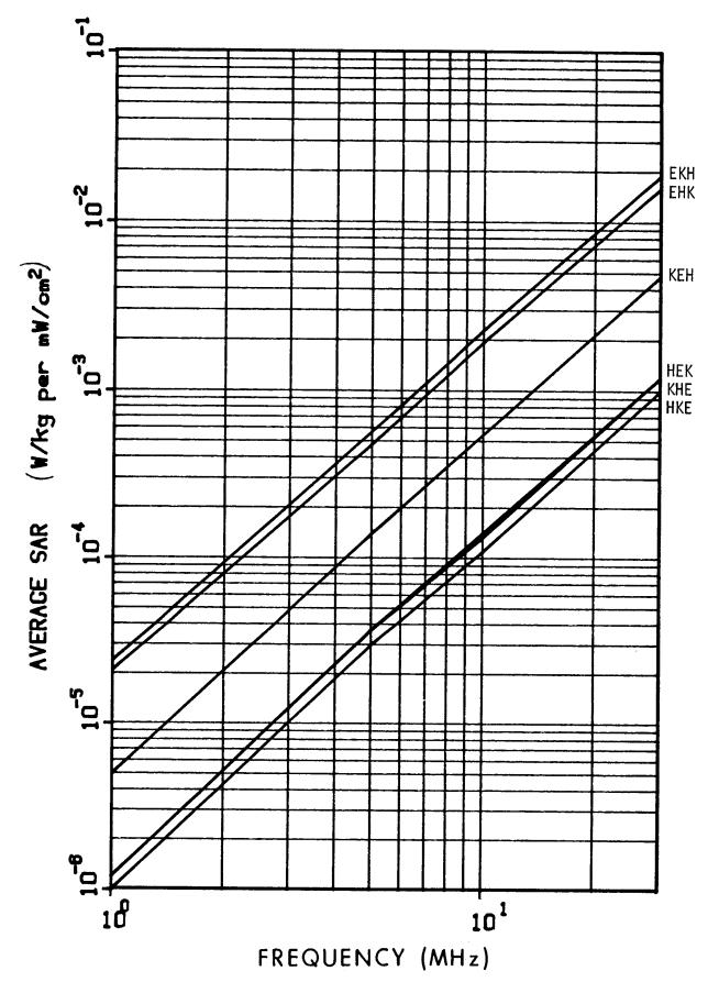
Figure 6.1. Calculated planewave average SAR in an ellipsoidal model of an average man, for the six standard polarizations; a = 0.875 m, b = 0.195 m, c = 0.098 m,  $V = 0.07 \text{ m}^3$ .
