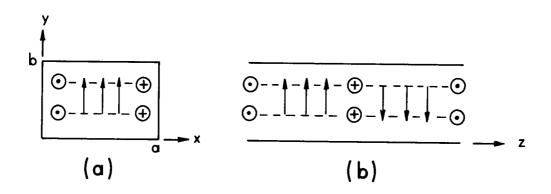
Figure 3.25. Field variation of the TE<sub>10</sub> mode in a rectangular waveguide (a) as would be seen looking down the waveguide and (b) as seen looking at the side of the waveguide. The solid lines are electric field and the dotted lines are magnetic field.
