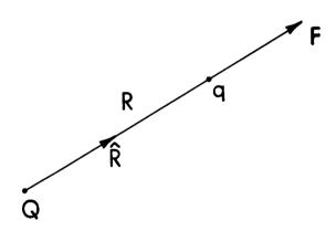
Figure 3.7. Force on a charge, q, due to the presence of another charge, Q.
