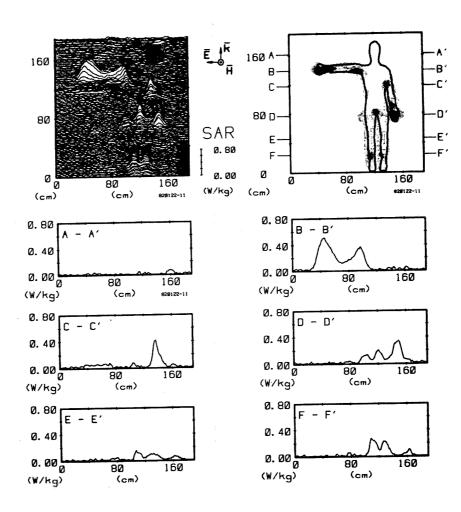
Figure 8.42. Computer-processed upper-body thermograms expressing SAR patterns for man with one arm extended, exposed to 1-mW/cm<sup>2</sup> 450-MHz radiation with KEH polarization (Guy et al., 1984) (© 1984 IEEE).
