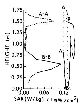
Figure 8.47. SAR distribution along an average man-model height for two cross sections; 1-mW/cm<sup>2</sup> incident-power density on the surface of the model, frequency 350 MHz E|L, K back to front (Krazewski et al., 1984) (© 1984, IEEE).
