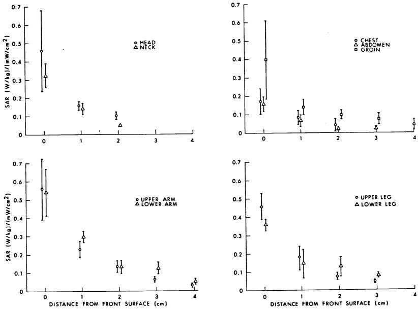
Figure 8.24. Normalized microwave absorption profiles in man-size model at 2.0 GHz. Vertical bars represent ±1 SD of the mean SAR. Minimum N, 3; average N, 5 (Olsen, 1982).
