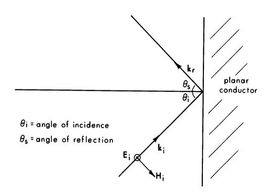
Figure 3.33. Planewave obliquely incident on a planar conductor.
