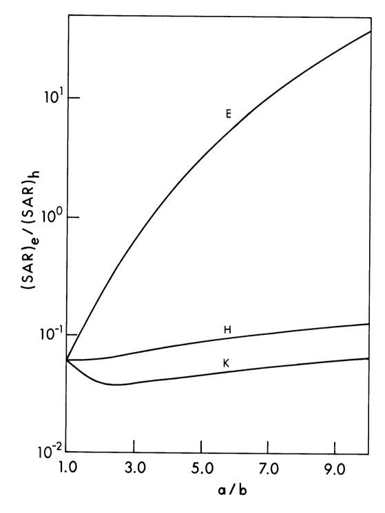
Figure 5.14. Ratio of  $(SAR)_e$  to  $(SAR)_h$  of a 0.07-m<sup>3</sup> prolate spheroid for each polarization as a function of the ratio of the major axis to the minor axis of the spheroid at 27.12 MHz,  $\sigma$  = 0.4 S/m.
