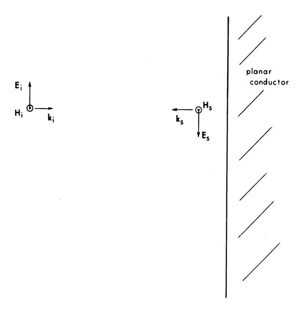
Figure 3.31. Planewave incident on a planar conductor.
