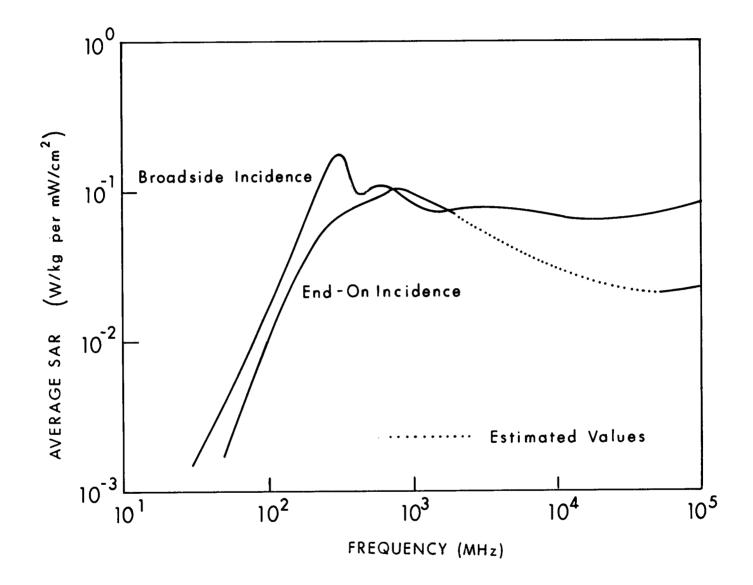
Figure 6.26. Calculated planewave average SAR in a prolate spheroidal model of a sitting rhesus monkey irradiated by a circularly polarized wave, for two polarized wave, b = 0.0646 m, V =  $3.5 \times 10^{-3}$  m<sup>3</sup>.
