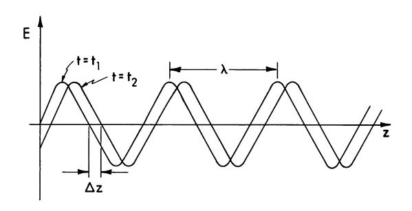
Figure 3.16. Snapshots of a traveling wave at two instants of time,  $t_1$  and  $t_2$ .
