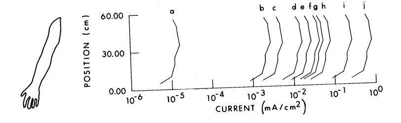
Figure 9.13. Calculated current density flowing through one arm. The exposure condition is the same as for Figure 9.12 (Guy and Chou, 1982).
