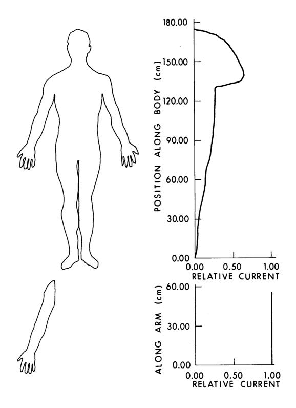
Figure 9.4. Relative surface-current distribution in man exposed to VLF-MF electric fields with feet insulated and hand grounded [after Deno, 1977 (Guy and Chou, 1982)].
