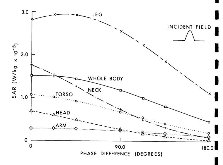
Figure 6.47. Whole- and part-body SAR at 77 MHz in the block model of man as a function of an assumed linear antisymmetric phase variation in the incident  $E_z$ ;  $E_z$  = 1 V/m. Calculated by Chatterjee et al. (1980a, 1980b, 1980c).
