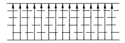
Figure 3.9. Field lines between infinite parallel conducting plates. Solid lines are E-field lines.
