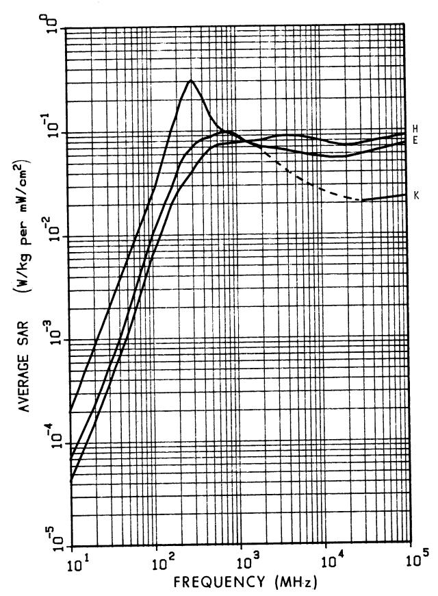
Figure 6.10. Calculated planewave average SAR in a prolate spheroidal model of a sitting rhesus monkey for three polarizations; a = 0.2 m, b = 0.0646 m,  $V = 3.5 \times 10^{-3} \text{ m}^3$ . The dashed line is estimated values.
