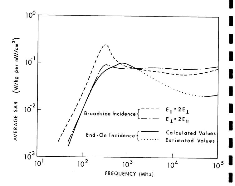
Figure 6.29. Calculated planewave average SAR in a prolate spheroidal model of a sitting rhesus monkey irradiated by an elliptically polarized wave, for two orientations; a = 0.2 m, b = 0.0646 m,  $V = 3.5 \times 10^{-3} \text{ m}^3$ .
