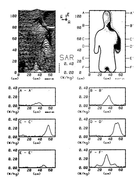
Figure 8.45. Computer-processed whole-body thermograms expressing SAR patterns for man sitting (frontal plane), exposed to  $1-mW/cm^2$  450-MHz radiation with EKH polarization (Guy et al., 1984) (© 1984 IEEE).
