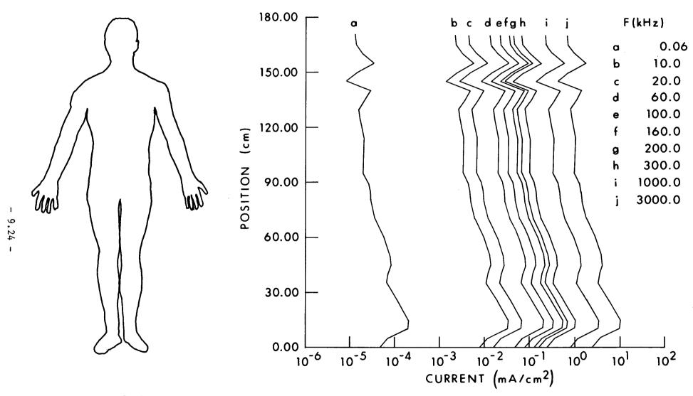
Figure 9.10. Calculated current distributions as a function of position in man exposed to 1-kV/m VLF-MF fields with feet grounded (Guy and Chou, 1982).
