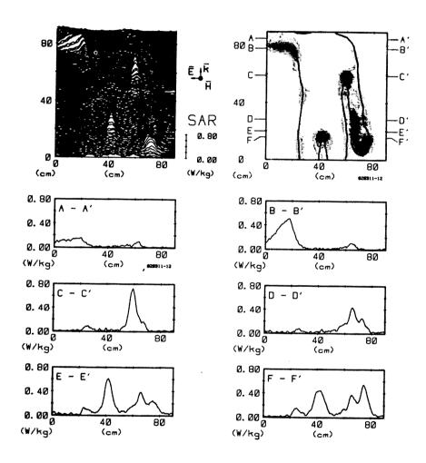
Figure 8.43. Computer-processed midbody thermograms expressing SAR patterns for man with one arm extended, exposed to 1-mW/cm<sup>2</sup> 450-MHz radiation with KEH polarization (Guy et al., 1984) (© 1984 IEEE).
