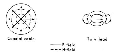
Figure 3.21. Cross-sectional views of the electric- and magnetic-field lines in the TEM mode for coaxial cable and twin lead.
