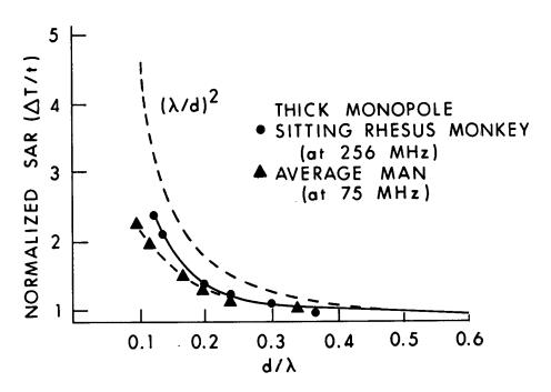
Figure 8.20. Measured relative SARs in scaled saline spheroidal models versus distance. SAR values for the different models are normalized with respect to their planewave value.  $\Delta T$  is the temperature rise in the saline solution after exposure for time t (Iskander et al., 1981).
