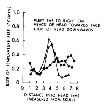
Figure 8.26. Rate of temperature rise from RFR exposure at the right side of a detached M. mulatta head; 1.2 GHz, CW, 70 mW/cm<sup>2</sup>, far field (Burr and Krupp, 1980).
