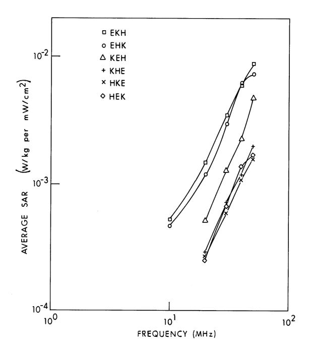
Figure 8.5. Measured values of the average SAR for saline-filled ellipsoidal phantoms, for six standard polarizations; a=20 cm, b=7.92 cm, c=5.28 cm,  $\sigma=0.64$  S/m (Allen et al., 1976).
