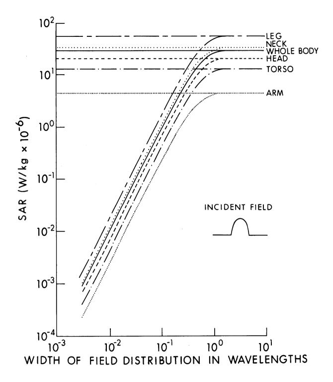
Figure 6.46. Average whole- and part-body SAR in the block model of man placed in front of a half-cycle cosine field,  $E_z$ ; frequency = 77 MHz,  $E_z$  = 1 V/m. Calculated by Chatterjee et al. (1980a, 1980b, 1980c).
