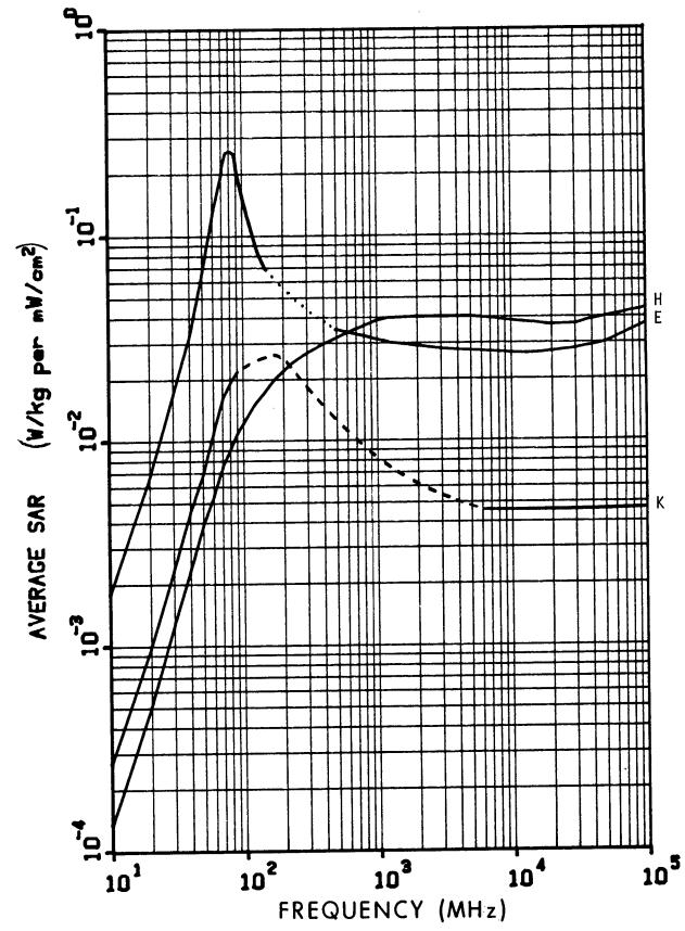
Figure 6.6. Calculated planewave average SAR in a prolate spheroidal model of an average woman for three polarizations; a=0.805 m, b=0.135 m, V=0.06114 m $^3$ . The dotted line is calculated from Equation 5.1; the dashed line is estimated values.
