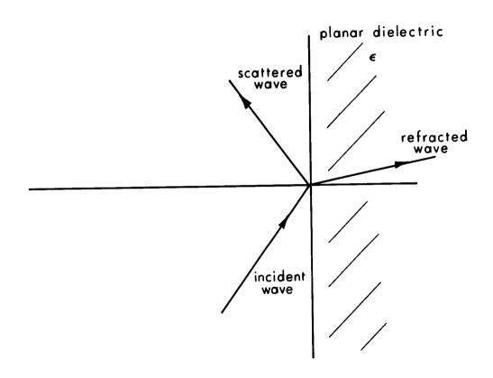
Figure 3.34. Planewave obliquely incident on a planar dielectric.
