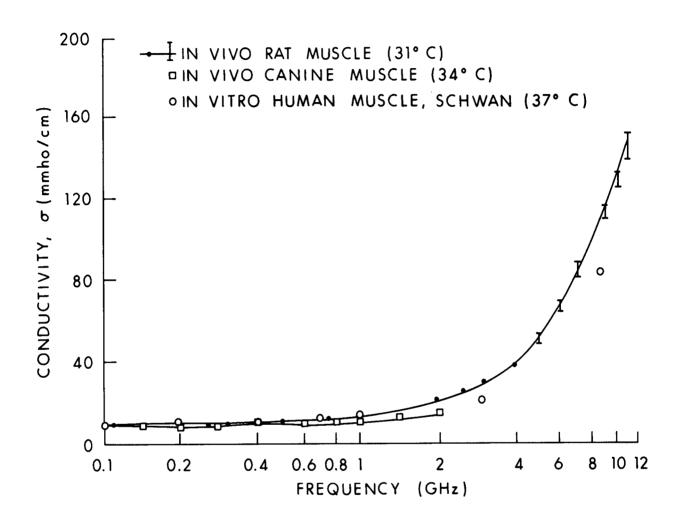
Figure 4.15. Measured values of conductivity of in vivo rat muscle and canine muscle (Burdette et al., 1980) compared to reference data (Schwan, 1957).
