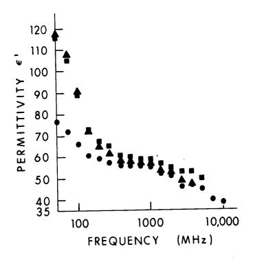
Figure 4.29. Real part of the dielectric constant, ε', of normal and tumor mouse tissue as a function of frequency (Rogers et al., 1983).
