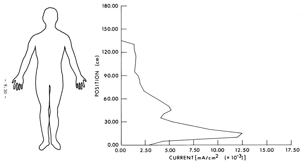
Figure 9.16. Calculated current distribution as a function of position in man with hand contacting a large object and with feet grounded. A 1-mA current is assumed to be flowing through the arm, thorax, and legs of the subject to ground,  $F = 60 \, \text{Hz}$  (Guy and Chou, 1982).
