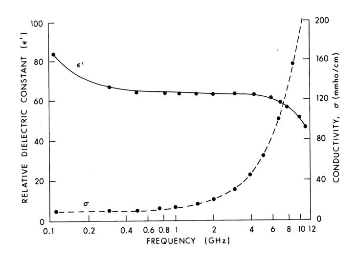
Figure 4.19. Measured values of relative dielectric constant and conductivity of rat blood at 23°C (Burdette et al., 1980).
