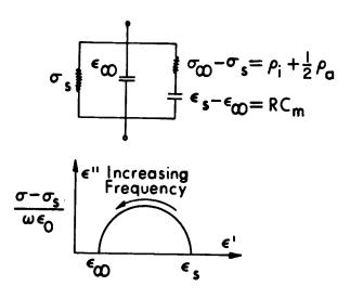
Figure 4.4. Equivalent circuit for the β-dispersion of a cell suspension and corresponding plot in the complex dielectric constant plane (Schwan and Foster, 1980).
