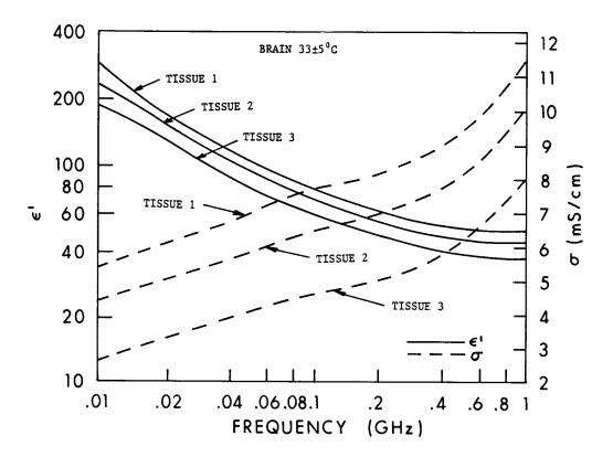
Figure 4.24. Relative permittivity of cat brain: tissue 1 -- gray matter; tissue 2 -- gray matter, 3 mm thick over white matter; tissue 3 -- white matter (Stuchly et al., 1981).
