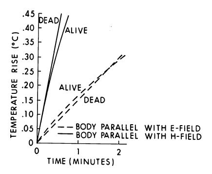
Figure 8.29. Temperature rise (at 2.0 cm into the top of the head) of an  $\underline{M}$ .  $\underline{\text{mulatta}}$  exposed to 70 mW/cm<sup>2</sup>, 1.2 GHz, CW, RFR, in the far field (Burr and Krupp, 1980).
