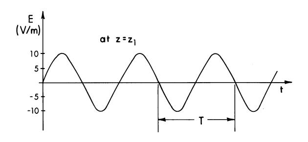
Figure 3.17. The variation of E at one point in space as a function of time.
