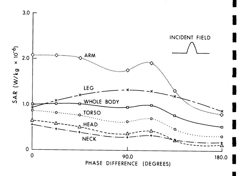
Figure 6.49. Whole- and part-body SAR at 350 MHz in the block model of man as a function of an assumed linear antisymmetric phase variation in the incident  $E_z$ ;  $E_z$  = 1 V/m. Calculated by Chatterjee et al. (1980a, 1980b, 1980c).
