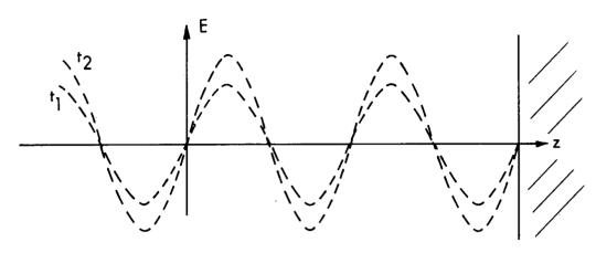
(a) Total  $\mathbf{E}$ -field as a function of position at two times,  $t_1$  and  $t_2$ .
