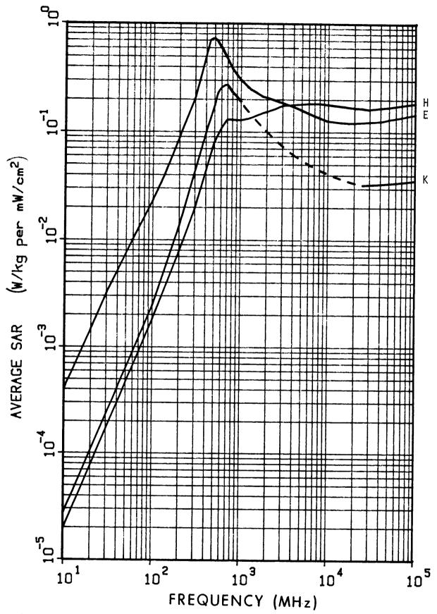
Figure 6.17. Calculated planewave average SAR in a prolate spheroidal model of a large rat for three polarizations; a = 0.12 m, b = 0.0322 m,  $V = 5.2 \times 10^{-4}$  m<sup>3</sup>. The dashed line is estimated values.
