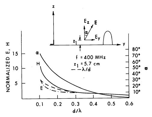
Figure 8.21. Measured relative fields versus distance for the thick monopole on a ground plane. The values of E and H are normalized with respect to their values at  $d/\lambda = 0.6$  (Iskander et al., 1981).
