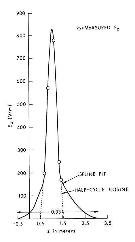
Figure 6.44. Incident-field  $\rm E_z$  from a 27.12-MHz RF sealer, used by Chatterjee et al. (1980a, 1980b, 1980c) in the planewave angular-spectrum analysis.
