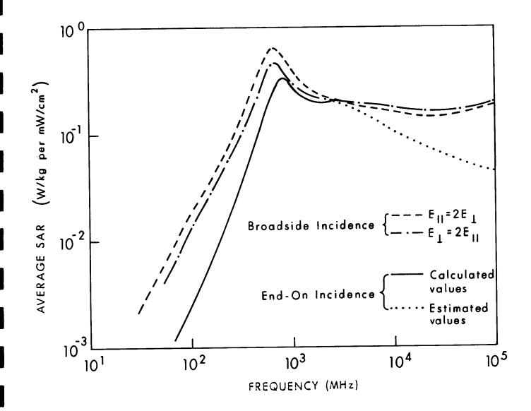
Figure 6.30. Calculated planewave average SAR in a prolate spheroidal model of a medium rat irradiated by an elliptically polarized wave, for two orientations; a = 0.1 m, b = 0.0276 m,  $V = 3.2 \times 10^{-4} \text{ m}^3$ .
