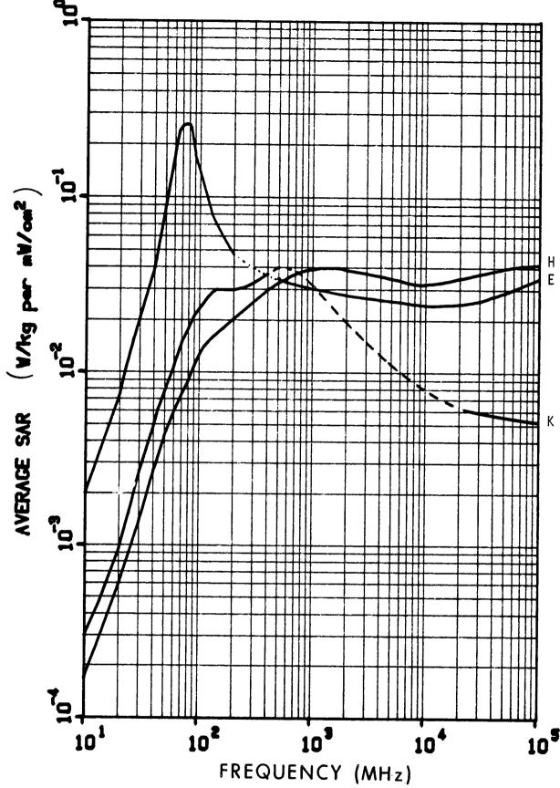
Figure 6.3. Calculated planewave average SAR in a prolate spheroidal model of an average man for three polarizations;  $a=0.875~m,\ b=0.138~m,\ V=0.07~m^3$ . The dotted line is calculated from Equation 5.1; the dashed line is estimated values.
