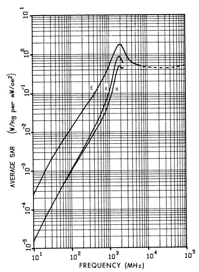
Figure 6.18. Calculated planewave average SAR in a prolate spheroidal model of a medium mouse for three polarizations; a=3.5 cm, b=1.17 cm, V=20 cm<sup>3</sup>. The dashed line is estimated values.
