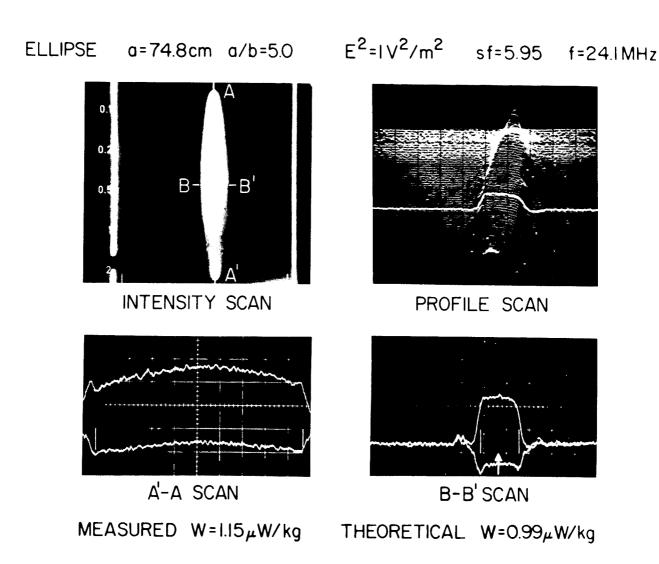
Figure 8.34. Scale-model thermograms and calculated peak SAR for 70-kg, 5/1 prolate spheroid (a = 74.8 cm) exposed to 24.1-MHz electric field parallel to the major axis: vertical divergence = 2°C, horizontal divergence = 2.65 cm (Guy et al., 1976b) (© 1976 IEEE).
