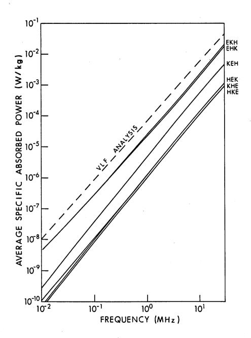
Figure 9.19. Comparison of calculated average SAR (obtained from VLF analysis) with average SAR (reported in the first edition of this handbook) of average absorbed power in an ellipsoidal model of an average man (Guy and Chou, 1982).
