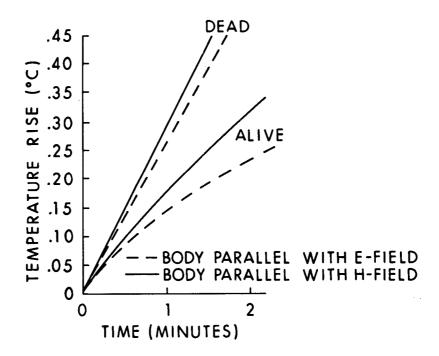
Figure 8.31. Temperature rise (at 3.5 cm into the back of the head) of an M. mulatta exposed to 70 mW/cm<sup>2</sup>, 1.2 GHz, CW, RFR, in the far field (Burr and Krupp, 1980).
