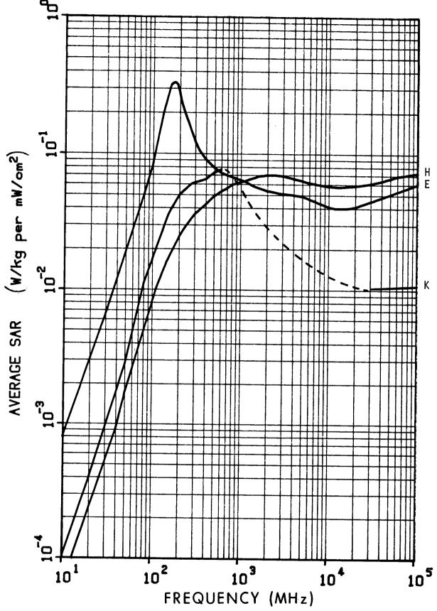
Figure 6.9. Calculated planewave average SAR in a prolate spheroidal model of a 1-year-old child for three polarizations; a=0.37 m, b=0.08 m,  $V=0.01 \text{ m}^3$ . The dashed line is estimated values.
