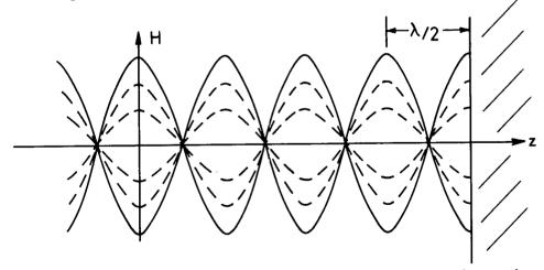
(c) Total H-field as a function of position at various times through a full cycle, and the envelope of the standing wave.
