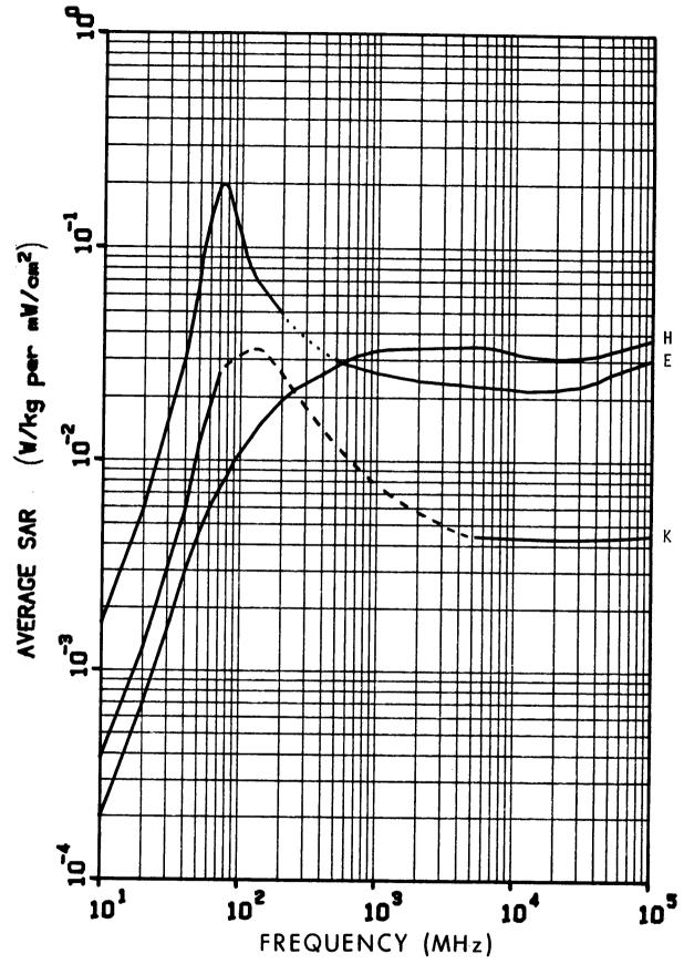
Figure 6.7. Calculated planewave average SAR in a prolate spheroidal model of a large woman for three polarizations; a=0.865 m, b=0.156 m,  $V=0.08845 \text{ m}^3$ . The dotted line is calculated from Equation 5.1; the dashed line is estimated values.
