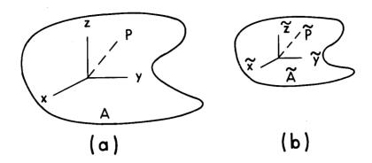
Figure 7.4. Schematic diagram illustrating the coordinate system used in the scaling procedure. (a) Full-size object with coordinate system x, y, z; (b) scaled model with coordinate system x, y, z.
