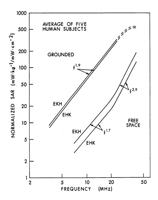
Figure 8.18. The frequency dependence of the average absorption rates for five human subjects in the EKH and EHK orientations under both free-space and grounded conditions (Hill, 1984).
