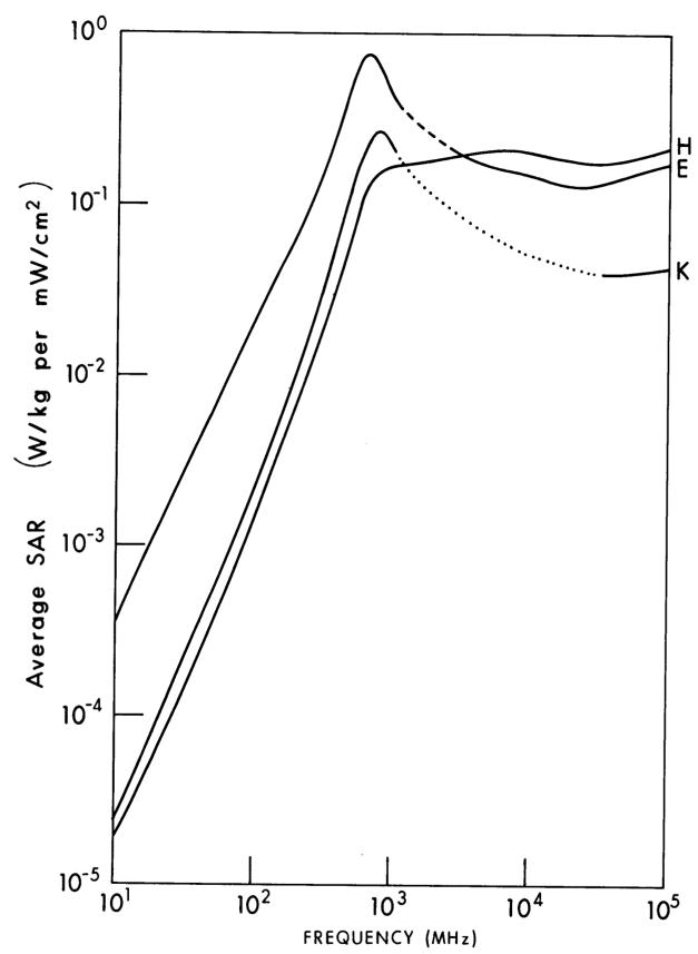
Figure 3.40. Calculated whole-body average SAR versus frequency for models of a medium-sized rat for three standard polarizations. The incident-power density is 1  $\rm mW/cm^2$ .
