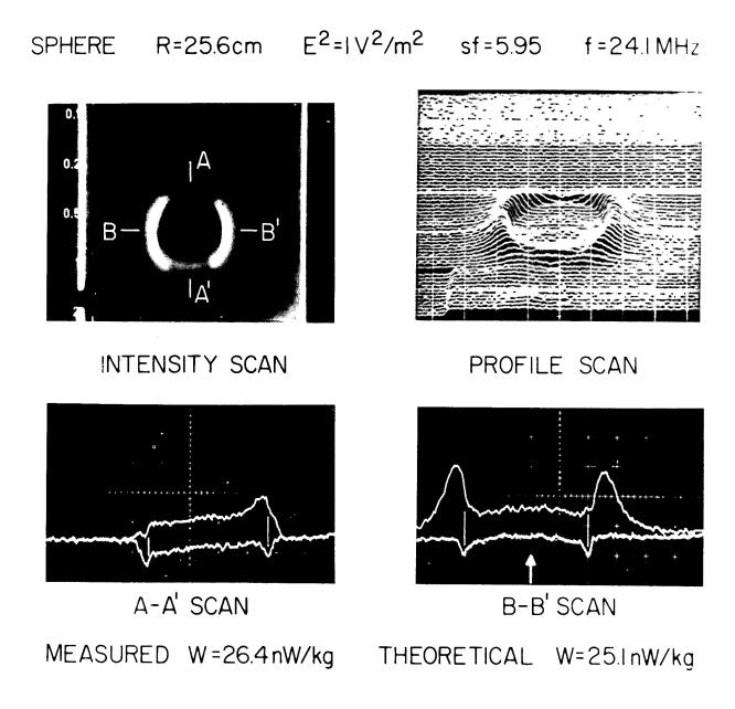
Figure 8.32. Thermographic results of exposing a 4.3-cm-radius sphere to 144-MHz TM<sub>110</sub> electric field in a rectangular resonant cavity simulating a 25.6-cm-radius sphere exposed to 24.1 MHz: vertical divergence = 2°C, horizontal divergence = 2 cm (Guy et al., 1976b) (© 1976 IEEE).
