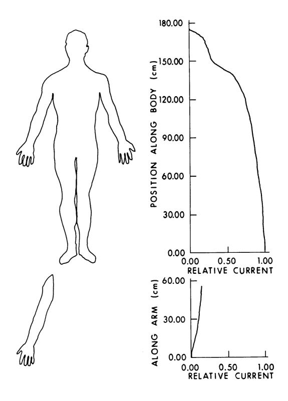
Figure 9.2. Relative surface-current distribution in grounded man exposed to VLF-MF fields [after Deno, 1977 (Guy and Chou, 1982)].
