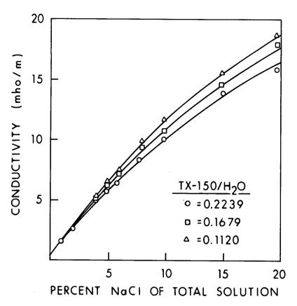
Figure 7.5. Electrical conductivity of phantom muscle as a function of NaCl and TX-150 contents measured at 100 kHz and 23°C.
