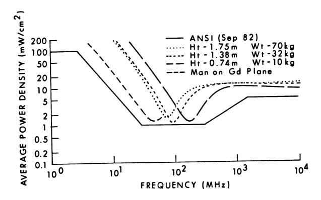
Figure 11.2. Power densities that limit human whole-body SAR to 0.4 W/kg compared to ANSI standard.
