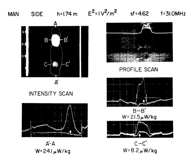
Figure 8.39. Scale-model thermograms and measured peak SAR for 70-kg, 1.74-m-height medial-plane man model exposed to 31.0-MHz electric field parallel to the major axis: vertical divergence = 2°C, horizontal divergence = 2.65 cm (Guy et al., 1976b) (© 1976 IEEE).
