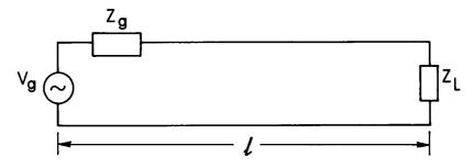
(b) Transmission line of length  $m{\ell}$  and load impedance  $Z_{m{L}}$
