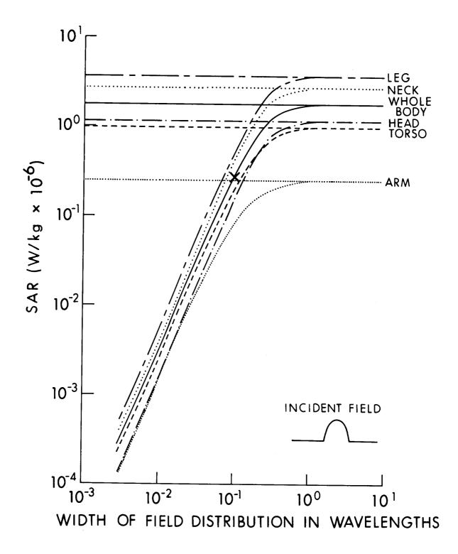
Figure 6.45. Average whole- and part-body SAR in the block model of man placed in front of a half-cycle cosine field,  $E_z$ ; frequency = 27.12 MHz,  $E_z$  = 1 V/m. Calculated by Chatterjee et al. (1980a, 1980b, 1980c).
