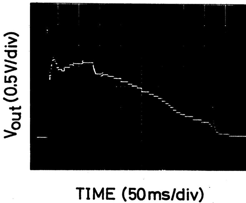
Fig.3 An example of the histogram obtained at the electron density measurement of JIPP T-II plasma.
