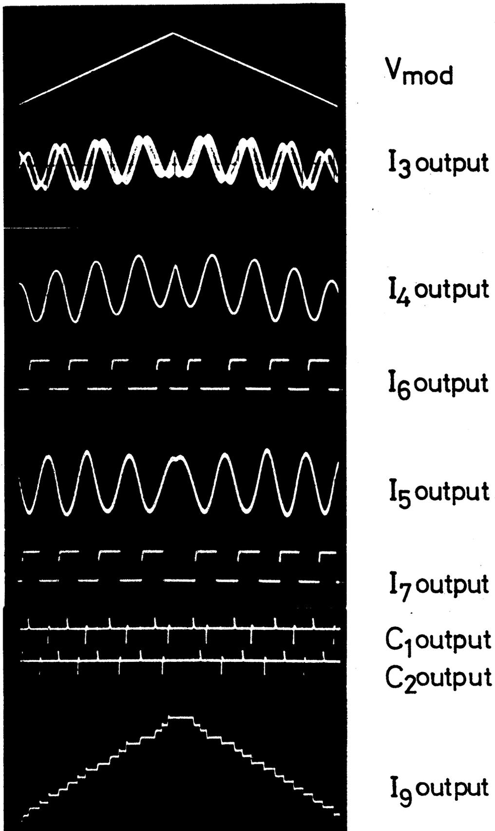
Fig.2 Oscillosgrams which show the relations between demodulated signals, outputs of the comparators, up- and down-pulses, and analog output, when the electron density evolution is simulated with triangular-wave modulation of the klystron frequency.
