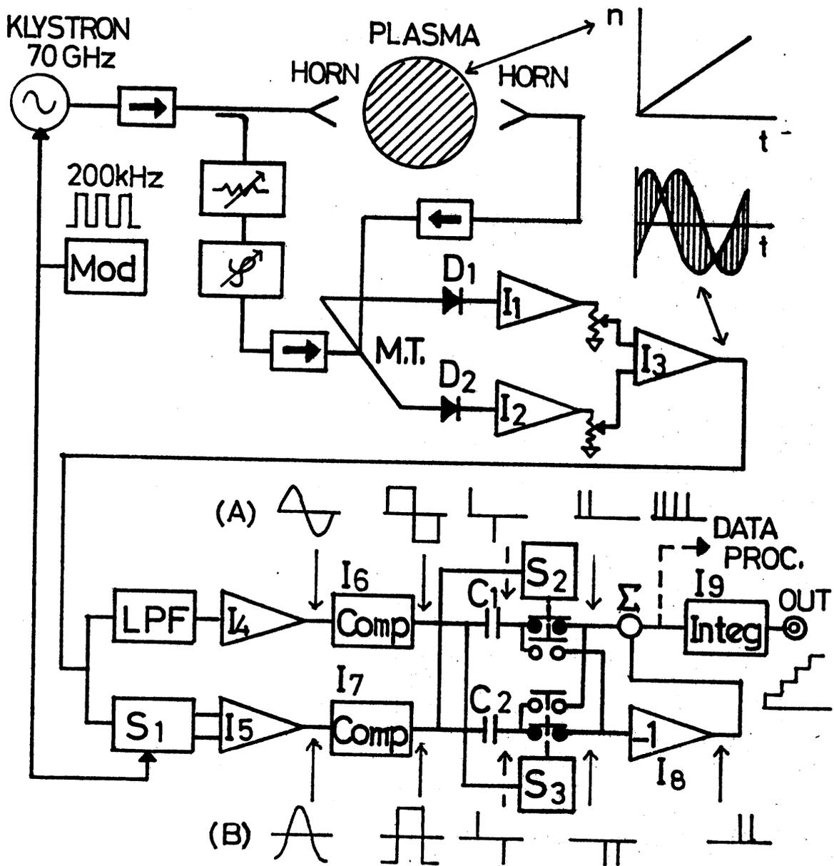
Fig.1 Schematic diagram of direct-reading type microwave interferometer. M. T.: magic-tee,  $D_1$ ,  $D_2$ : crystal detectors,  $I_1$ ,  $I_2$ ,  $I_3$ ,  $I_4$ ,  $I_5$ ,  $I_8$ : IC amplifiers,  $I_6$ ,  $I_7$ : comparators,  $I_9$ : integrator,  $S_1$ ,  $S_2$ ,  $S_3$ : analog switches, LPF: low pass filter. Waveforms to be observed for linearly increasing density are also shown.
