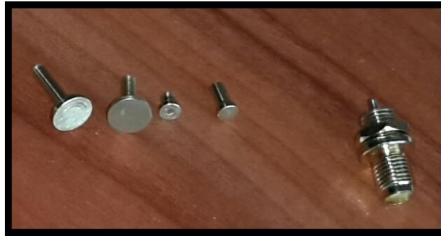
Figure 52. Part 4, unified antenna and exciting probe and part 5, SMA connector
