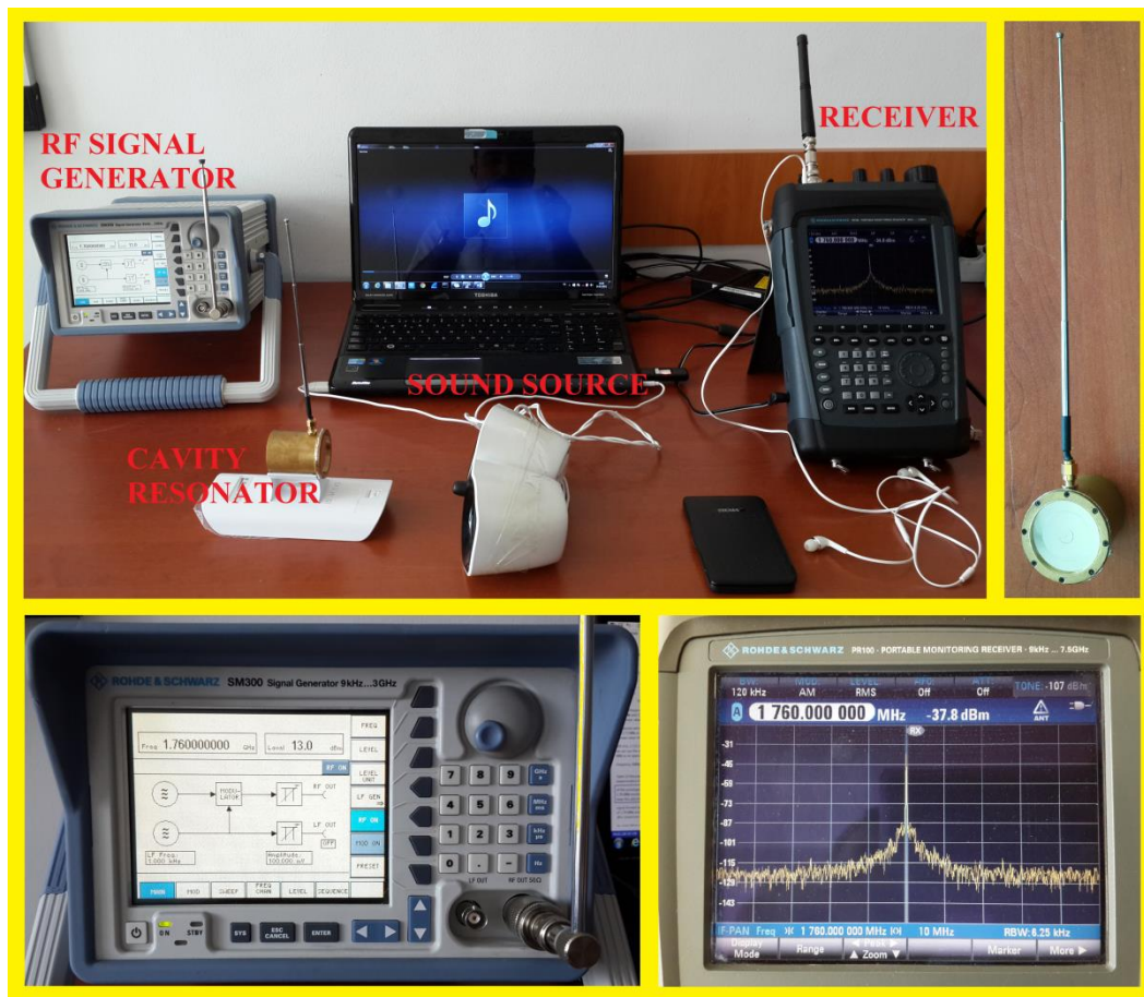
Figure 71. Sound receive experiment setup
