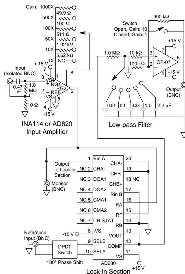
Figure 1. The schematic of the low-cost LIA. Only three integrated circuits are used. The values of the gain resistors shown are for the INA114. Each integrated circuit may be bypassed at its power supply terminals with 0.1  $\mu\text{F}$  capacitors, which are not shown in the schematic. The output can be conveniently read by a digital dc voltmeter.
