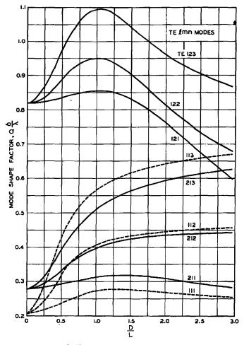
Fig. 4—Mode-shape factors  $\left( \frac{O}{\lambda} \right)$  as a function of diameter to length ratio  $\left( \frac{D}{L} \right)$  for circular cylinder resonator — TE modes with l > 0.
