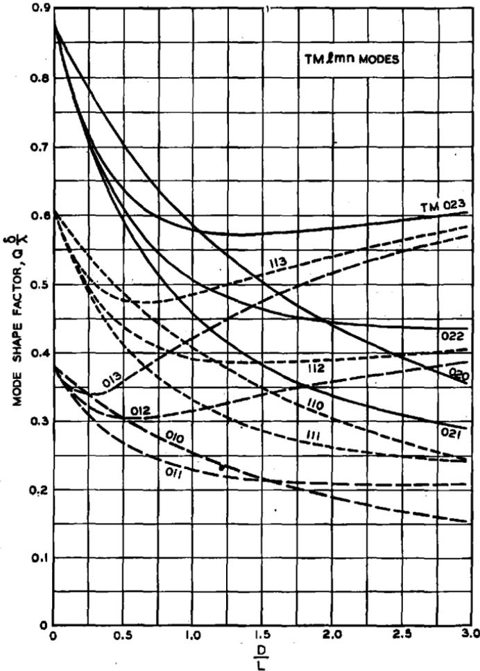
Fig. 2—Mode-shape factors  $(Q^{\delta}/\lambda)$  as a function of diameter to length ratio  $(D/L)$  for circular cylinder resonator—*TM* modes.
