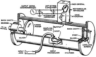
Fig. 9-Schematic of a 9 kmc echo box.
