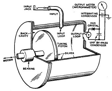
Fig. 8-Schematic of a 3 kmc echo box.
