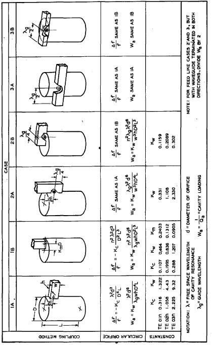
TABLE IV.—Orifice Coupling of Wove Guide (TE 10 Mode) to Cylindrical Cavity (TE 0mn Mode)
