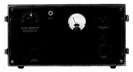
Fig. 14-Panel view of a 9 kmc echo box.
