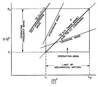
Fig. 5—Mode chart illustrating meaning of crossing and interfering modes and of operating area.
