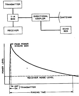
Fig. 10-Radar test with echo box.
