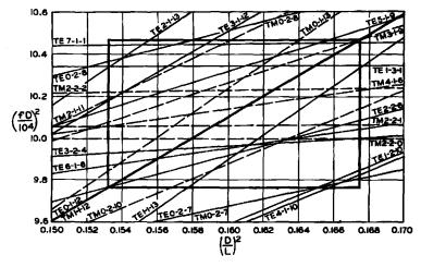
Fig. 7—Expanded mode chart covering the operating area of a 9 kmc echo box.
