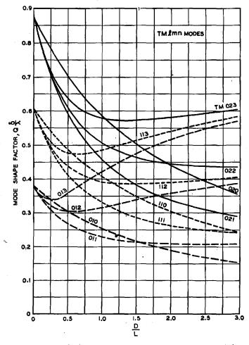
Fig. 2—Mode-shape factors  $\left(Q^{\delta}_{\lambda}\right)$  as a function of diameter to length ratio  $\left(\frac{D}{L}\right)$  for circular cylinder resonator—TM modes.
