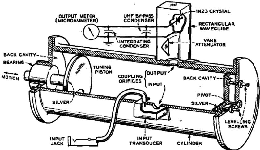
Fig. 9—Schematic of a 9 kmc echo box.
