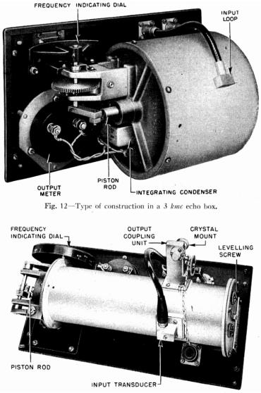
Fig. 13-Type of construction in a 9 kmc echo box.
