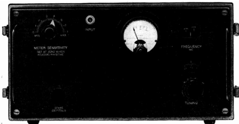
Fig. 14—Panel view of a 9 kmc echo box.
