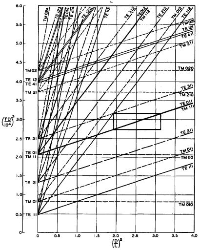
Fig. 1-Mode chart for right circular cylinder resonant cavity.
