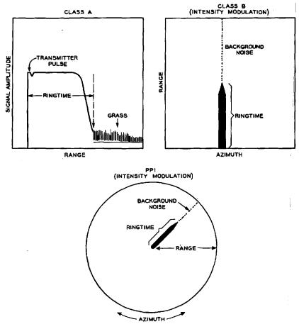
Fig. 11.—Typical ringtime patterns on radar indicators.
