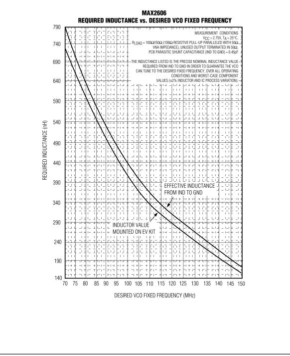
Figure 2. MAX2606 Required Inductance vs. Desired VCO Fixed Frequency
