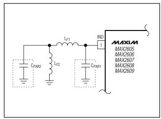
Figure 7. Simple Model of External Inductance
