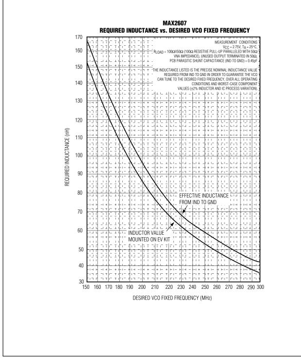
Figure 3. MAX2607 Required Inductance vs. Desired VCO Fixed Frequency
