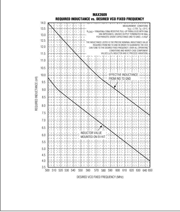
Figure 5. MAX2609 Required Inductance vs. Desired VCO Fixed Frequency
