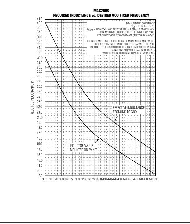
Figure 4. MAX2608 Required Inductance vs. Desired VCO Fixed Frequency
