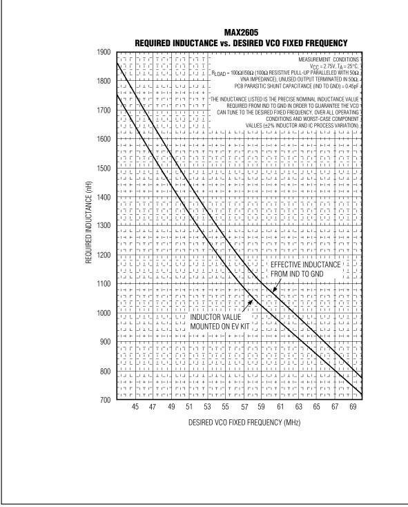
Figure 1. MAX2605 Required Inductance vs. Desired VCO Fixed Frequency
