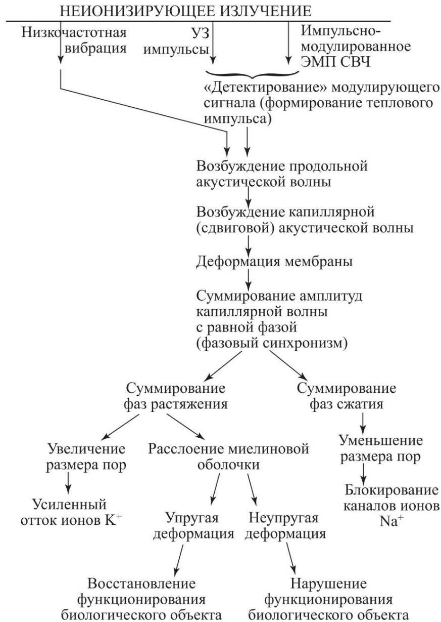
Rice. 3.07. Scheme for converting the absorbed energy of a non-ionizing radiation
