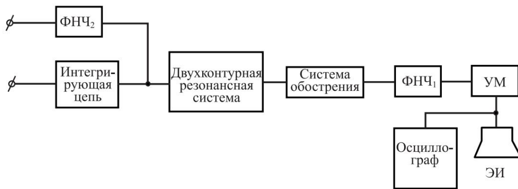
Rice. 4.34. Block diagram of the electrical model: 1 - low-pass filter (LPF2), 2 - integrating circuit, 3 - double-circuit resonant system, 4 — aggravation system, 5 — low-pass filter (LPF1), 6 — amplifier power, 7 - oscilloscope, 8 - electrodynamic emitter
