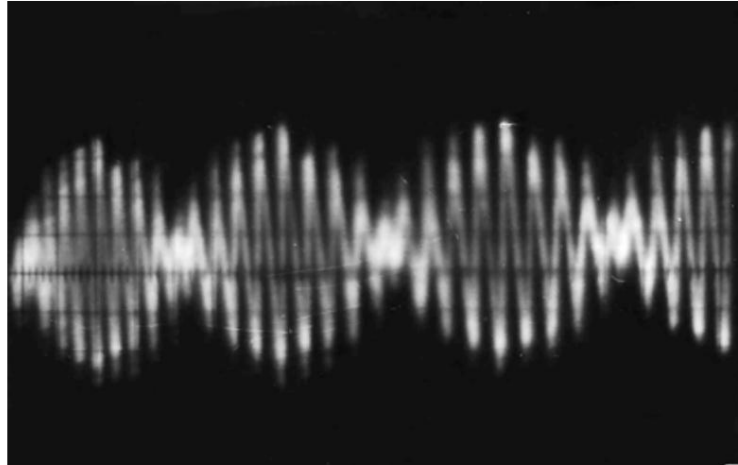
Rice. 2.16. Oscillogram of zero beats excited in ethyl alcohol mechanical vibrations and acoustic sinusoidal signal
