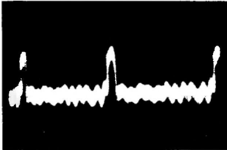
Rice. 32. Damping of excited mechanical vibrations in ethanol
