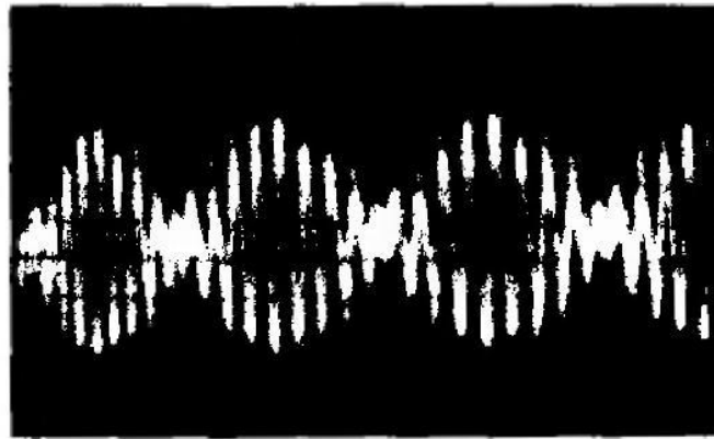
Rice. 29. Beating of mechanical vibrations excited in a test tube by EMR pulses with an acoustic signal
