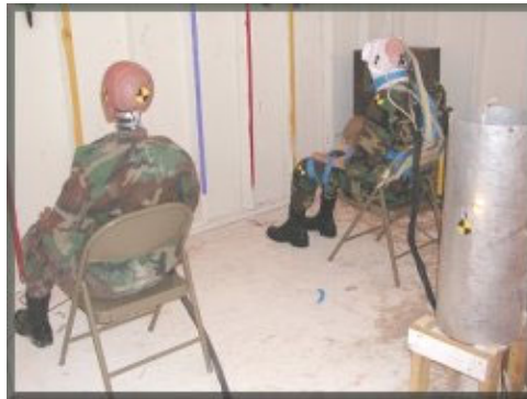
Pre-test Anthropomorph and Cadaver Setup Inside a SEA Hut
