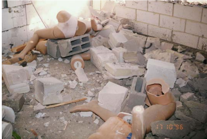
Figure 30: CMU Debris Impact on Mannequins
