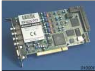
Fig. 5 4-channel, 20 kHz (per channel) PCI- based DSP (FFT) card ZD0860
