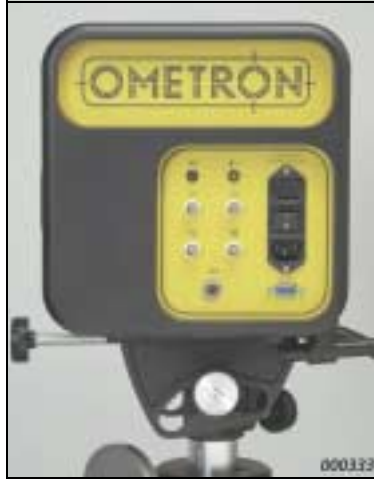
Fig. 10 Sensor Head SB2507 showing side-panel with connectors
