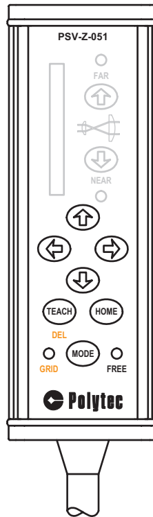
Figure 5.3: Defining and deleting scan points using the hand set PSV-Z-051
