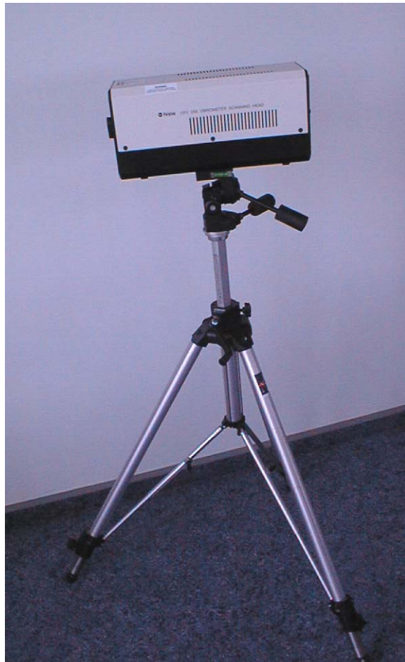
Figure 3.11: Scanning head mounted on the fluid stage and on the tripod
