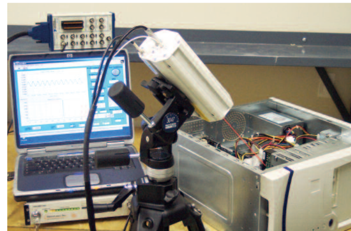
Computer Components Measuring vibration of a computer disk drive.
