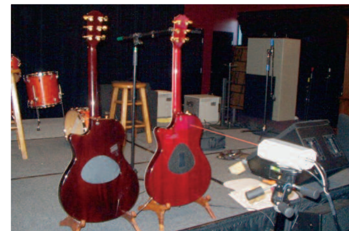
Musical Instruments Measuring acoustic decay time of identical guitars made from different wood.
