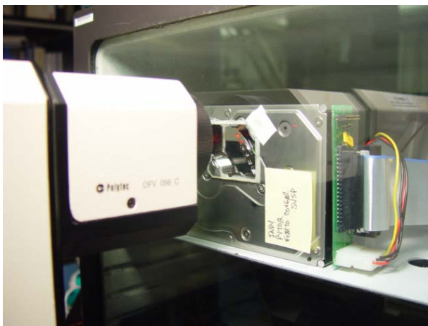
Figure 13: PSV measuring file in vacuum chamber
