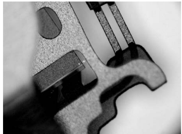
Figure 14. Laser beam of an MSV measuring a location on the slider TE
