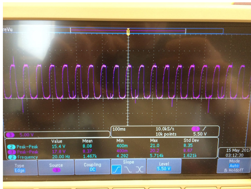
Figure 18: Output From the Full Bridge Class D with a Sine Wave Input
