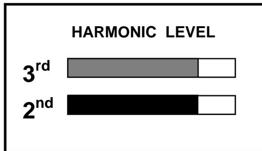
Both meters show a strong return. This indicates a corroded junction because of the high level of 3<sup>rd</sup> harmonic.
