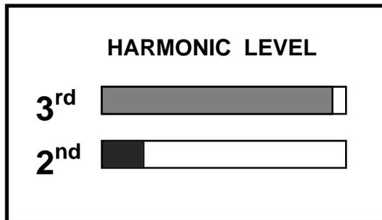
High 3<sup>rd</sup> harmonic level indicates corroded metallic junction
