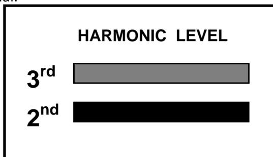
Both meters are full scale. The operator can not tell which is the stronger signal.
