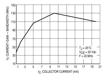
Figure 3. Current-Gain — Bandwidth
