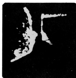
b. TURN VR3 CW TO CORRECT. Straight target appears bent inward at the screen center.
