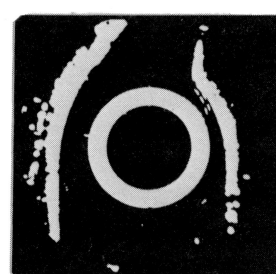
c. TURN VR3 CCW TO CORRECT. Straight target appears bent outward at the screen center.
