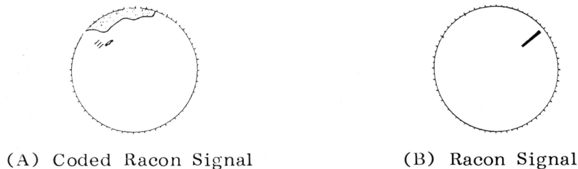
Fig.41 Racon Signal Appearance
