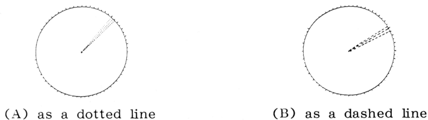
Fig.42 Ramark Signal Appearance
