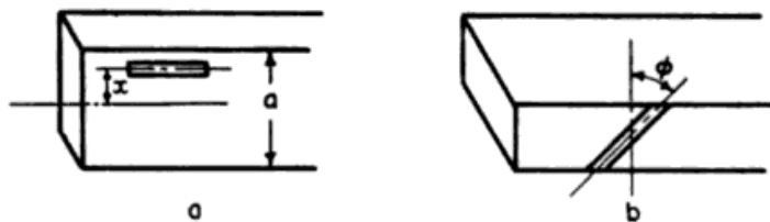
Figure 164.—(a) and (b) show how the coupling of a shunt slot to a waveguide may be varied by either displacing it towards the centre of the broad face of the guide or by suitably orienting it in the narrow face.
