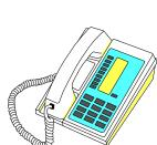
handset and the ringing element of a telephone. They can easily be activated by signals unintentionally emitted from RED/BLACK equipment. These signals can be picked up and transmitted by a telephone, even when the phone is on hook.
