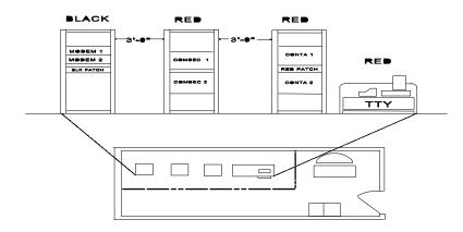
Figure 2-1, Non-TEMPEST Approved Equipment Spacing
