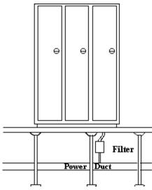
example of where BLACK power filters are normally installed. Consult your project package for specific filter locations.
