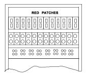
personnel. As shown in the adjacent figure, different types of RED patch jacks are installed to prevent physical connection between different communities or classifications of security.
