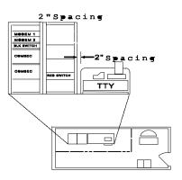
practices such as minimum cable bending radius of the sizes of interconnecting ducts and conduits. The separation distance cannot be less than that established IAW RED/BLACK <u>standards</u> listed in MIL-HDBK-232A, Table 11, NACSIM 5203, Table 3-1, and applicable CM tables in AFSSI 7002. Improper spacing distances could result in a TEMPEST hazard.
