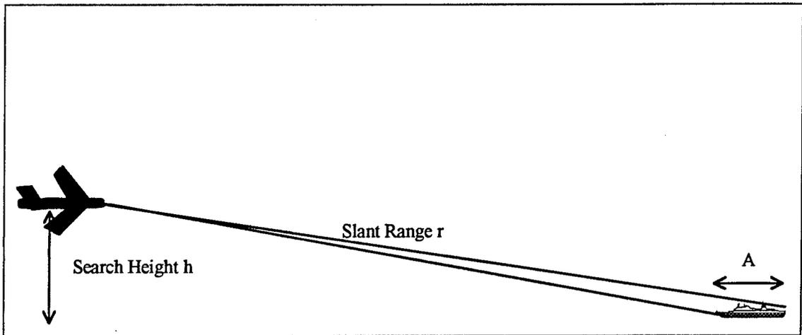
Figure 17: Relationship of  $h$ ,  $r$  and  $A$  in Pollock detection rate model
