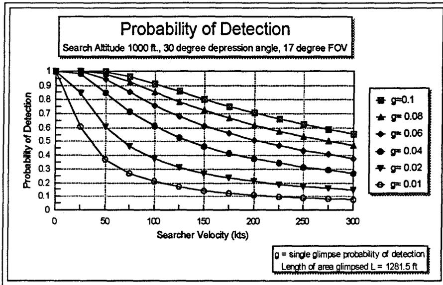
Figure 15: Probability of detection with 17° FOV
