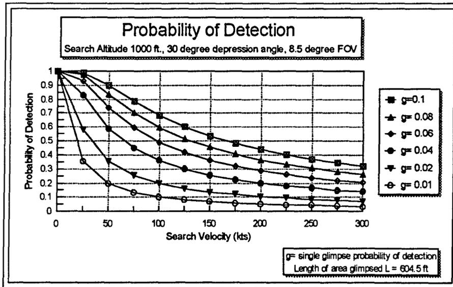
Figure 16: Probability of detection with 8.5° FOV
