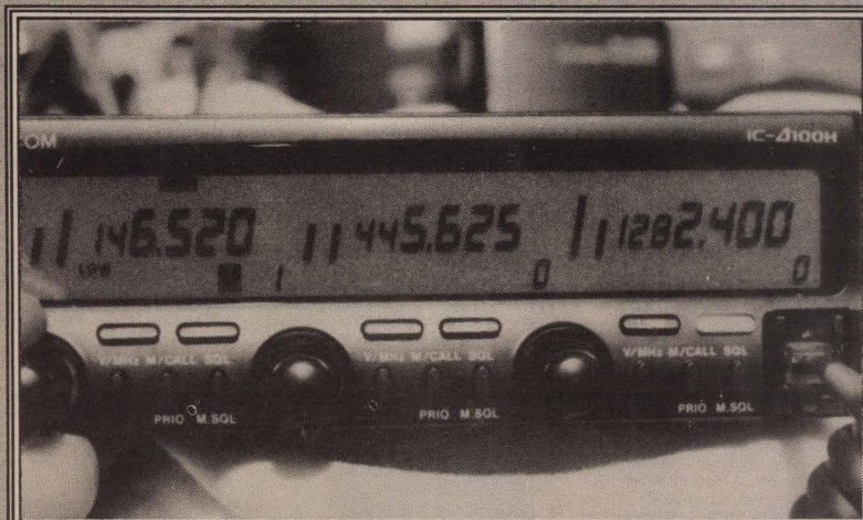
This Icom transceiver is capable of tri-band cross-band operation.
