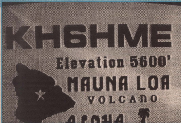
2,700 mile TV reception from Hawaii to California on 434 MHz. Tropospheric ducting made it all possible!
