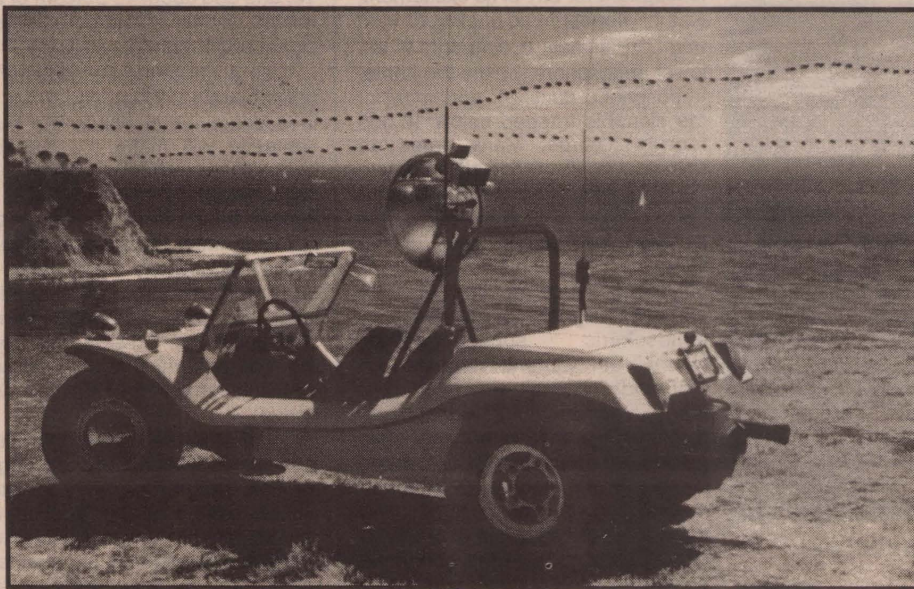
Perfect microwave tropo weather for author West and his mobile 10 MHz station. (Dotted lines show tropo duct.)
