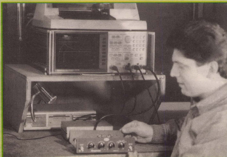
Technician tuning a new band- pass filter system.
