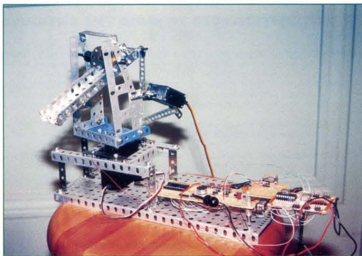
Photos 12a,b (top and bottom, respectively) — Two views of a tilt/pan/zoom web cam platform that I built.
