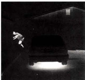
An Indigo Systems Merlin infrared camera shows car in the road ahead (note hot area of exhaust system) and a pedestrian outside the headlight beam. Photo courtesy of Indigo Systems.
