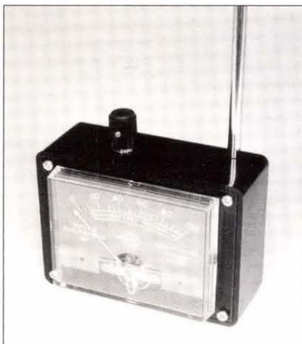
The completed RF Meter sensitivity is controlled by a top-mounted knob.
