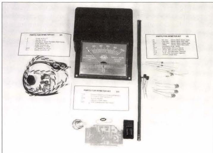
Every part needed is furnished with the RF Meter Kit from LNS Technologies.
