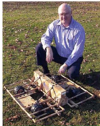
The Mine Rover, developed at Johns Hopkins University's Applied Physics Laboratory, provides sophisticated, inexpensive mine detection. Photo courtesy of Johns Hopkins APL.
