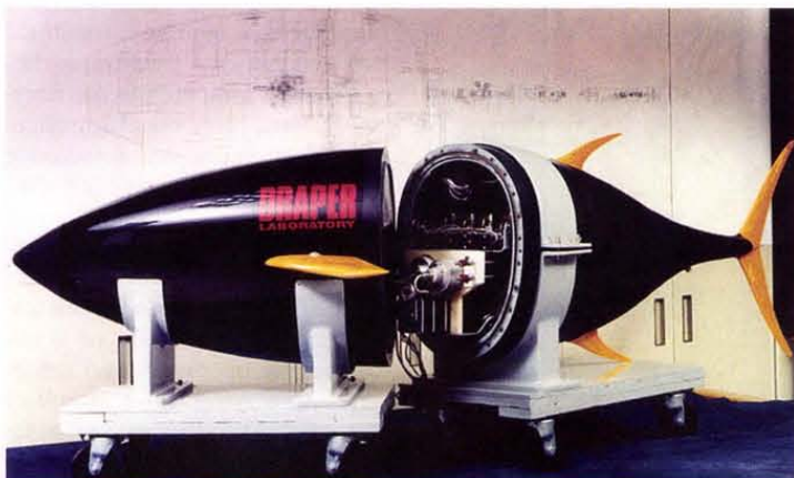
Draper's "Robotuna" may have applications in undersea exploration, clearing mines, and laying cable. Source: The Charles Stark Draper Laboratory, Inc., Cambridge, MA, USA.
